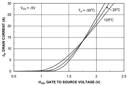
Figure 5. Transfer Characteristics.
