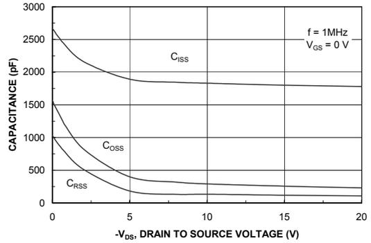
Figure 8. Capacitance Characteristics.
