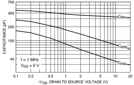
Figure 8. Capacitance Characteristics.
