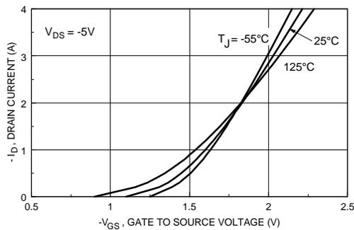
Figure 5. Transfer Characteristics.
