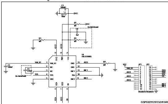
Figure 1: STEVAL-MKI166V1 board schematic
