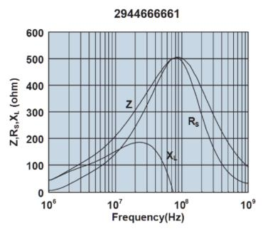
Impedance, reactance, and resistance vs. frequency.
