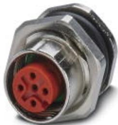
Sensor/actuator flush-type socket, 5-pos., M12 SPEEDCON, A-coded, rear/screw mounting with Pg9 thread, with 0.5 m TPE litz wire, 5 x 0.34 mm<sup>2</sup>
