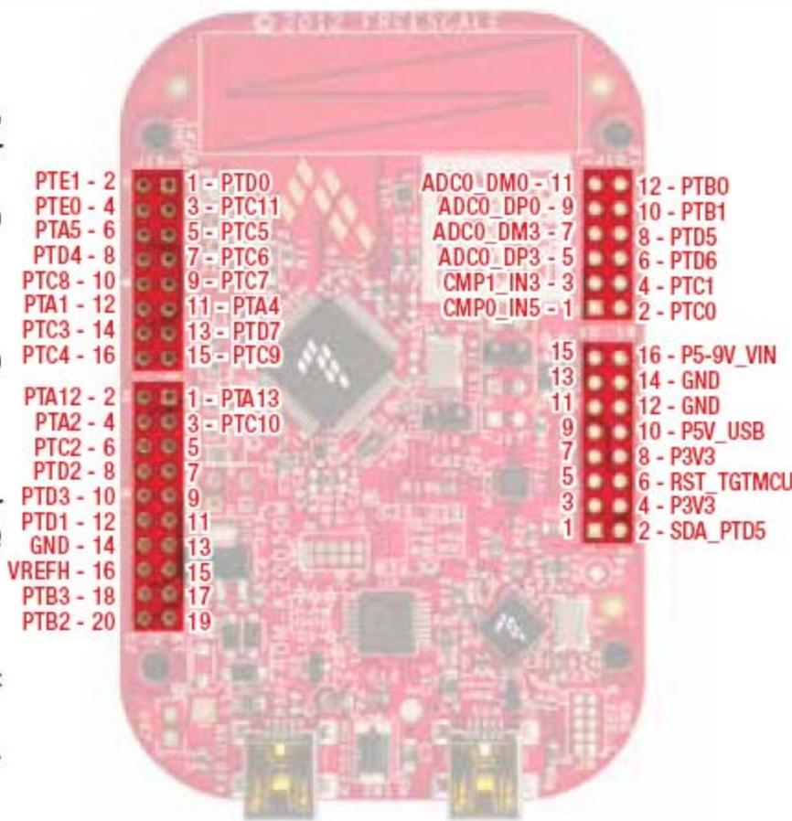
Figure 2: FRDM-K20D50M Pin-Out
