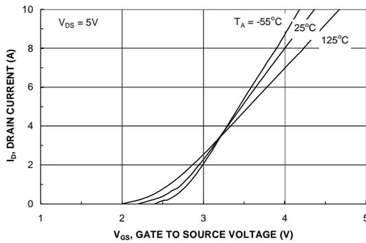
Figure 5. Transfer Characteristics.
