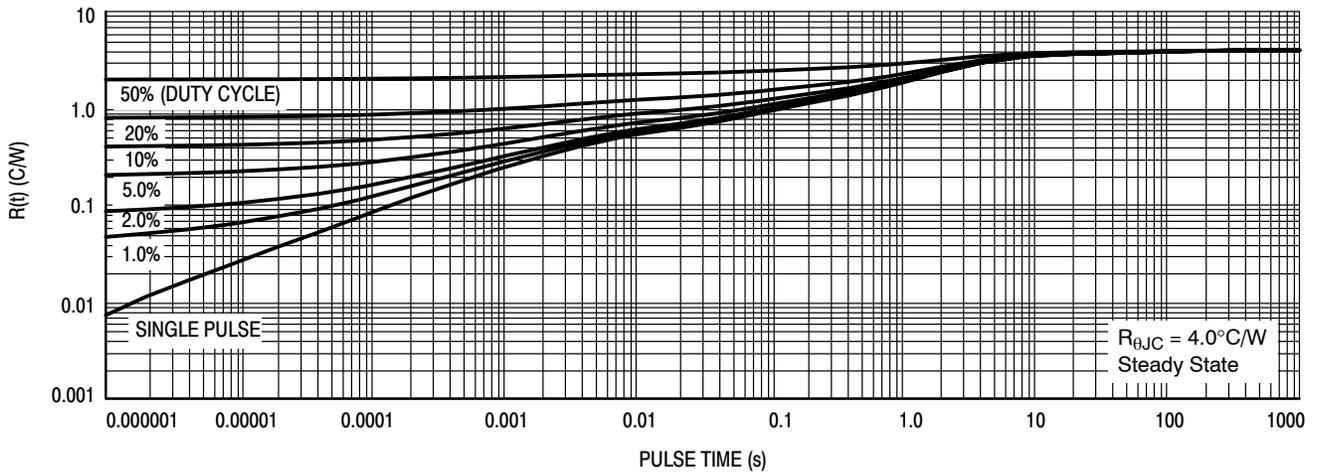
Figure 13. Thermal Impedance for NDF06N62Z
