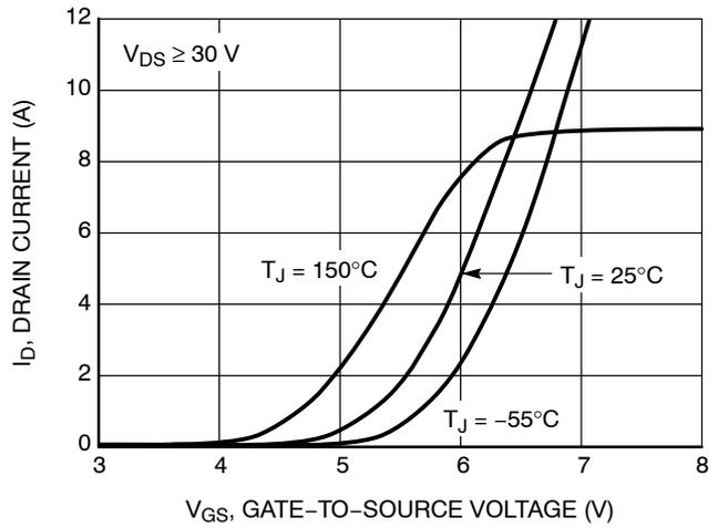
Figure 2. Transfer Characteristics
