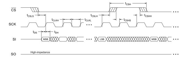
Figure 14-2. Serial Output Timing
