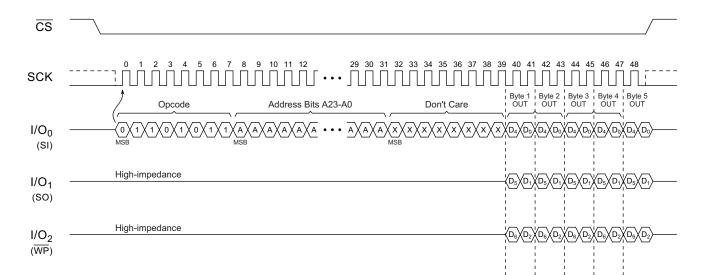
Figure 7-5. Quad-Output Read Array
