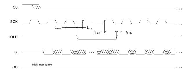
Figure 14-5. HOLD Timing – Serial Output
