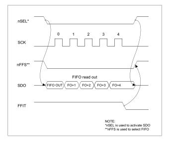
During FIFO access the  $f_{sck}$  cannot be higher than  $f_{ref}/4$ , where  $f_{ref}$  is the crystal oscillator frequency.
