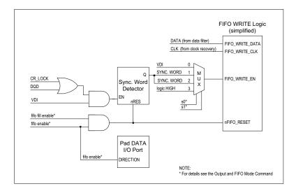
Note: VDI (Valid Data Indicator) see further details in Receiver Control Word, Synchron word in microcontroller mode is 2DD4h.
