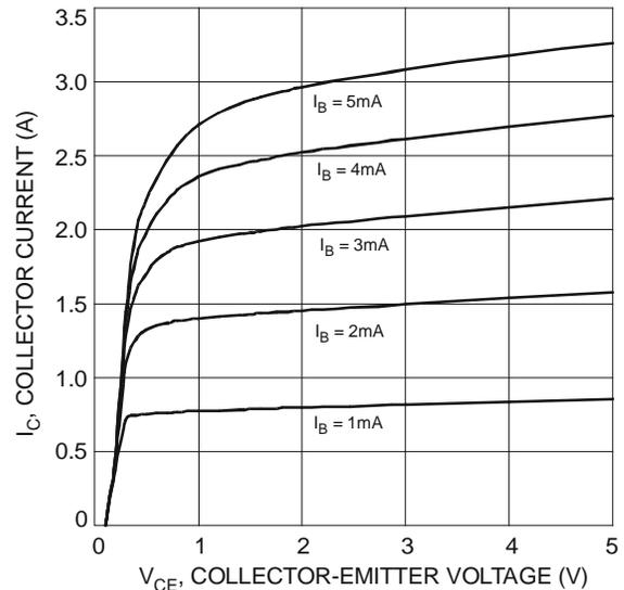
Fig. 2 Typical Collector Current vs. Collector-Emitter Voltage
