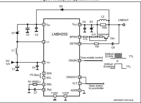
Figure 7: DiSEqC 2.x application circuit
