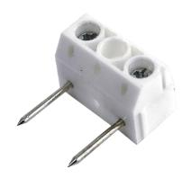
LED's **Solderless** Inspired 2-Prong Screw Terminal pairs with our Infinity Series Weather Resistant LED Dura-flex, terminating bare ends to cable. Sturdy prongs pierce the copper wiring on either side of flex to create a secure connection. while screw terminals allow cable to be run from strip to strip, or directly to power source.
