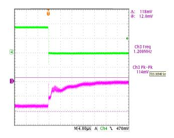
FIGURE 4. FALLING EDGE TRANSIENT RESPONSE
