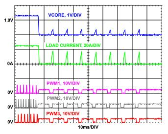
FIGURE 5. OVERCURRENT PROTECTION
