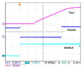
FIGURE 2. SOFT-START INTERVAL WAVEFORMS
