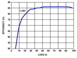
FIGURE 8. VRM EFFICIENCY vs LOAD CURRENT
