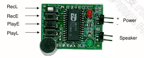
**Power**: Make sure the polarity is connecting correctly or the board will be damaged. The input voltage can be ranging from 2.4 to 5.5V.
