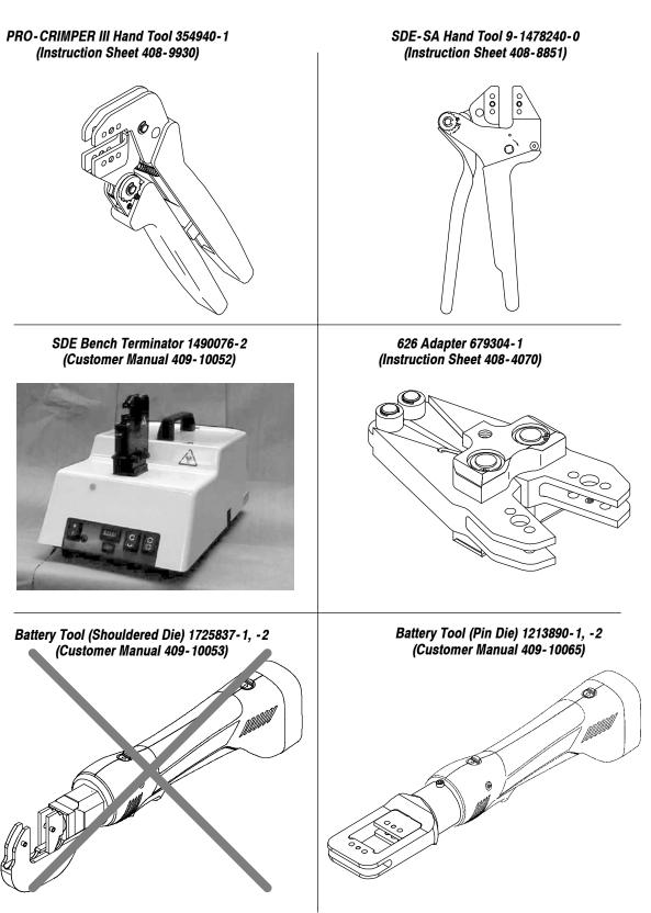
Tooling Compatible with Die Assembly 2063820-2
