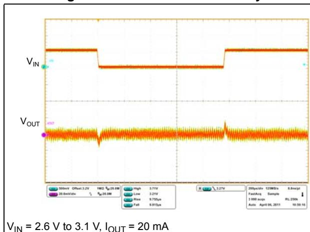
$V_{IN} = 2.6\text{ V to }3.1\text{ V}$ ,  $I_{OUT} = 20\text{ mA}$
