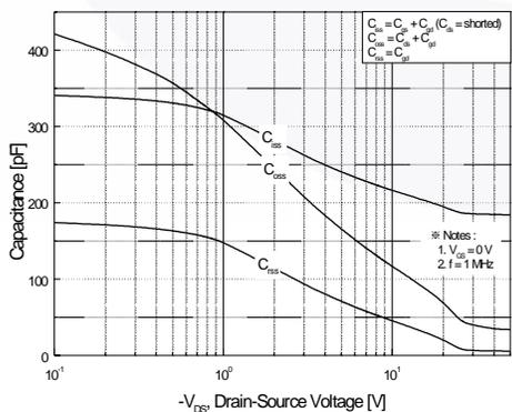
Figure 5. Capacitance Characteristics
