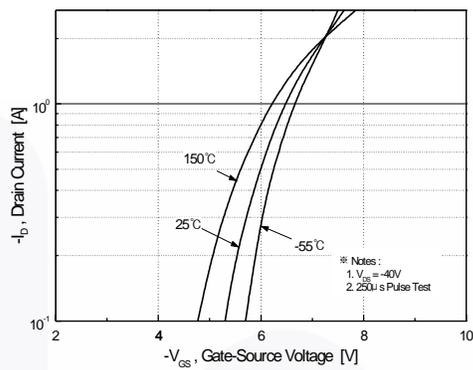
Figure 2. Transfer Characteristics
