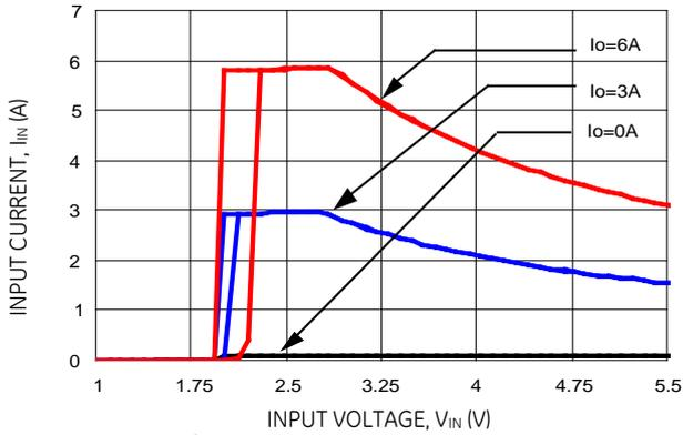
**Figure 7. Input voltage vs. Input Current**
