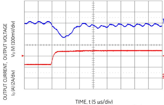
**Figure 10. Transient Response to Dynamic Load Change**
