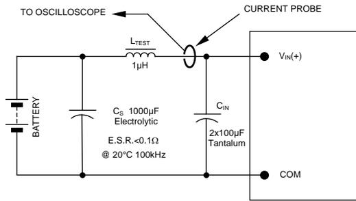
NOTE: Measure input reflected ripple current with a simulated source inductance (L<sub>TEST</sub>) of 1µH. Capacitor C<sub>S</sub> offsets possible battery impedance. Measure current as shown above.
