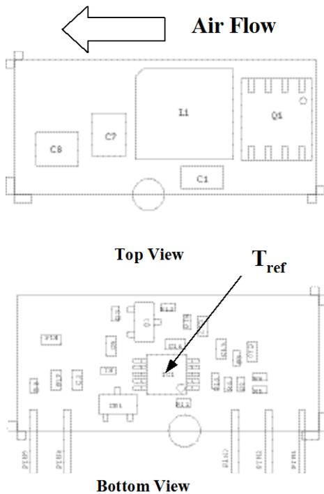
Figure 33. Thermal Test Set-up.
