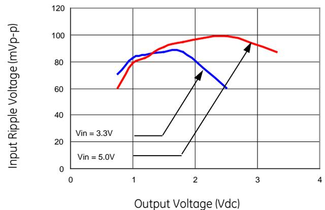
Figure 26. Input ripple voltage for various output with 1x150 µF polymer and 1x47 µF ceramic capacitors at the input (80% of I<sub>o,max</sub>).
