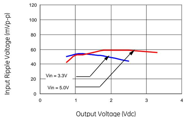
Figure 27. Input ripple voltage for various output with 2x150 µF polymer and 2x47 µF ceramic capacitors at the input (80% of I<sub>o,max</sub>).
