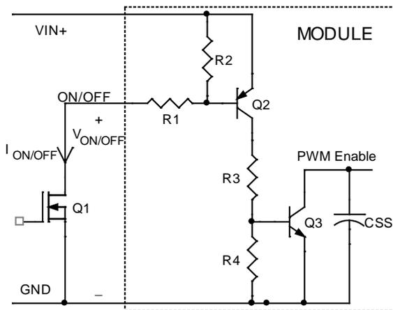
**Figure 28. Circuit configuration for using positive logic On/Off.**
