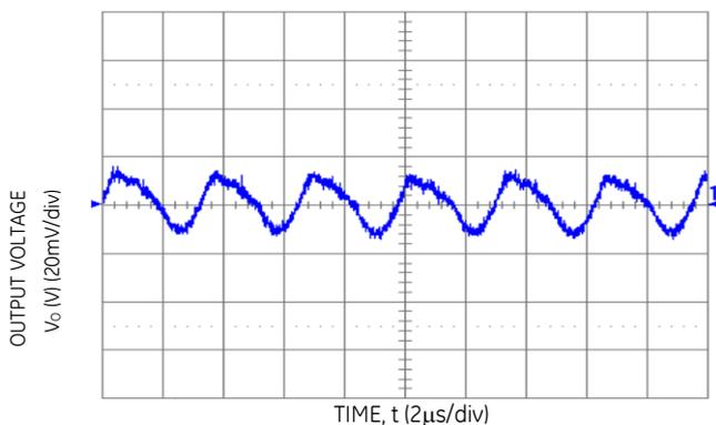
**Figure 9. Typical Output Ripple and Noise**
