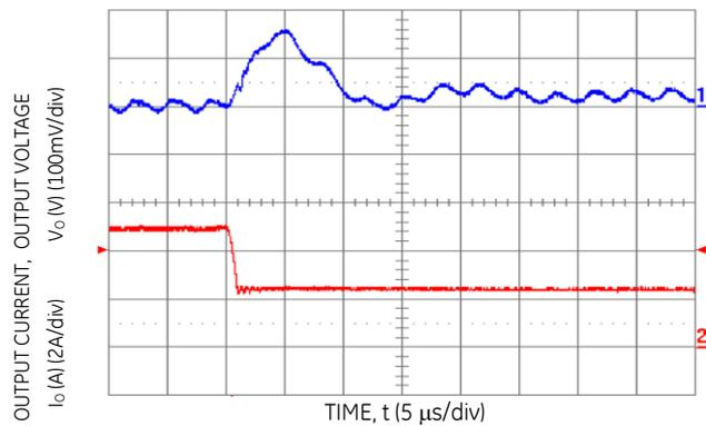
**Figure 11. Transient Response to Dynamic Load Change**
