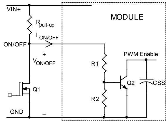
**Figure 29. Circuit configuration for using negative logic On/Off.**
