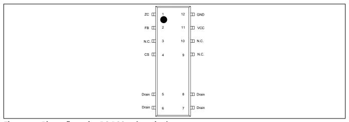
Figure 2 Pin configuration PG-DSO-12(top view)
