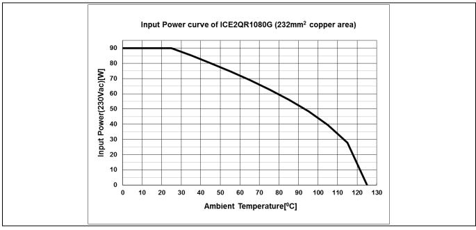
Input power curve V<sub>IN</sub>=230 V<sub>AC</sub>; P<sub>in</sub>=f(T<sub>a</sub>) Figure 14
