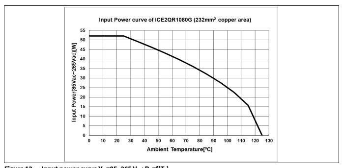
Input power curve V<sub>IN</sub>=85~265 V<sub>AC</sub>; P<sub>in</sub>=f(T<sub>a</sub>) Figure 13
