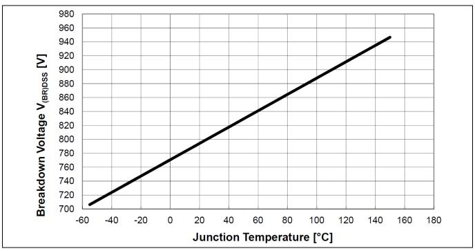
Figure 12 Drain-source breakdown voltage;  $V_{BR(DSS)}=f(T_i)$ ,  $I_D=0.25mA$
