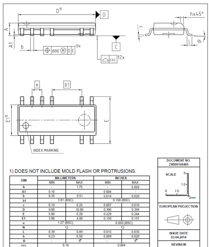
Figure 15 PG-DSO-12 (Pb-free lead plating Plastic Dual-in-Line Outline)
