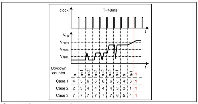
Figure 6 Up/down counter operation
