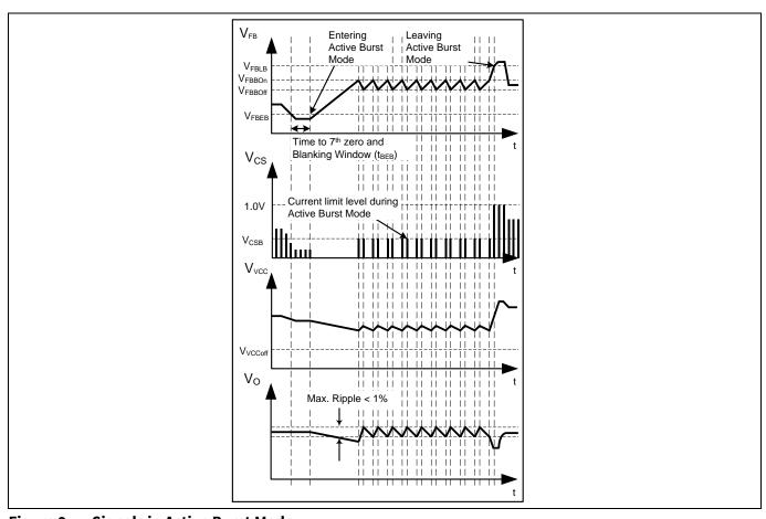
Figure 9 Signals in Active Burst Mode
