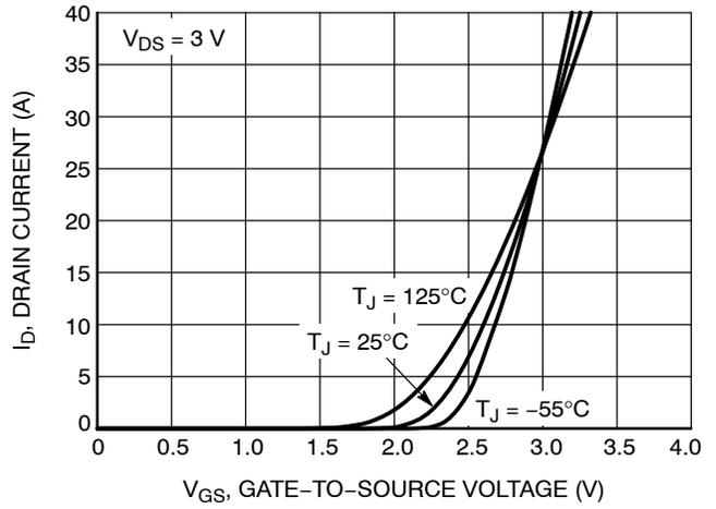
Figure 2. Transfer Characteristics
