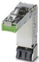
RJ45 connector, Degree of protection: IP20, Number of positions: 8, Material: Zinc die-cast, Connection method: IDC, Connection cross section: AWG 23-22, Cable exit: angled, High degree of resistance to vibration; 360° shielding; one-piece design; special tool-free assembly
