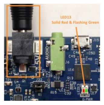
3) Connect the USB cable provided with the DK-S3A7 to the J-Link OB (J15) on the Main Board.
