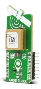
**GNSS 4 click** carries SAM-M8Q patch antenna module from u-blox. The click is designed to run on a 3.3V power supply. It communicates with the target microcontroller over I2C or UART interface.
