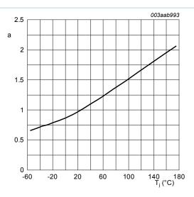
Fig. 17. Normalized drain-source on-state resistance factor as a function of junction temperature
