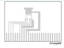
Fig. 7. PCB used for thermal tests; zero heat sink area
