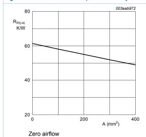
Fig. 6. Thermal resistance from junction to ambient as a function of printed-circuit board (PCB) heat sink area
