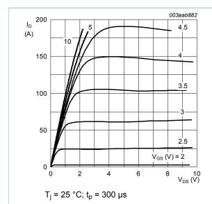
Fig. 10. Output characteristics; drain current as a function of drain-source voltage; typical values
