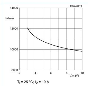
Fig. 18. Ratio of drain current to sense current as a function of gate-source voltage; typical values
