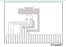
Fig. 8. PCB used for thermal tests; heat sink area 200 mm<sup>2</sup>
