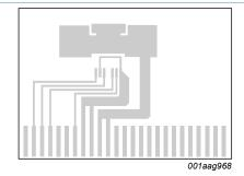
Fig. 9. PCB used for thermal tests; heat sink area 400 mm<sup>2</sup>
