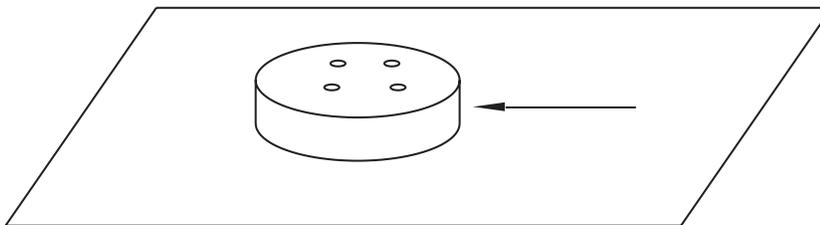
Note: 1. When soldered to PCB, must have >10 N resistance to horizontal loading.
