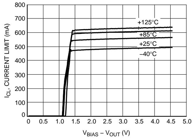
Figure 10. Current Limit vs. ( $V_{BIAS} - V_{OUT}$ )
