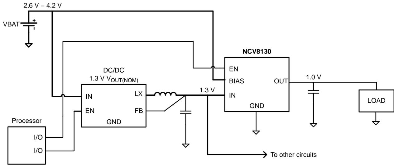
Figure 3. Typical Application: Low-Voltage Post-Regulator with ON/OFF functionality
