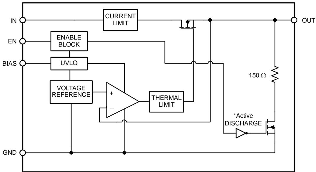
\*Active output discharge function is present only in NCV8130AMXyyyTCG devices.
