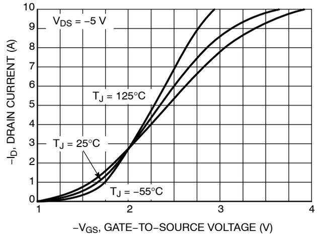
Figure 2. Transfer Characteristics
