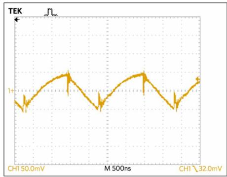
Figure 3. Output ripple at 800mA load, 12Vout.
