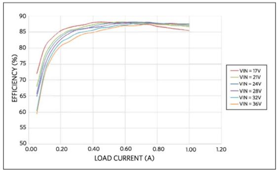
Figure 2. Power efficiency vs. load current.
