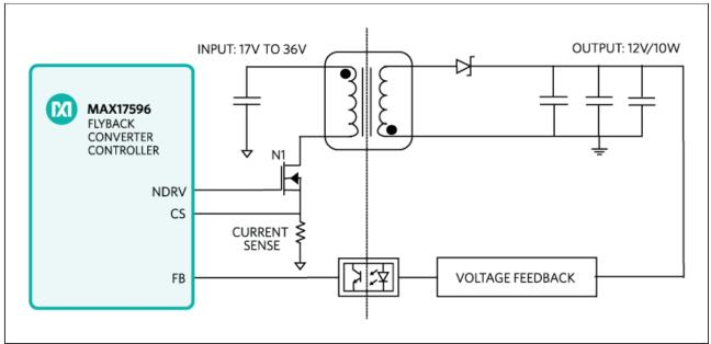
Figure 1. MAXREFDES112# block diagram.
