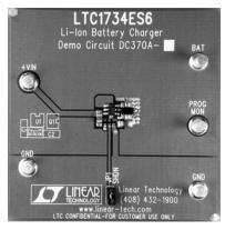
Other Features include;Preset float voltages of 4.1 & 4.2V ±1%<br/>700mA Constant Current (can be programmed for other charge<br/>currents ranging from 100mA to 700mA)<br/>Monitor charge current using the Program pin<br/>No isolation diode required
