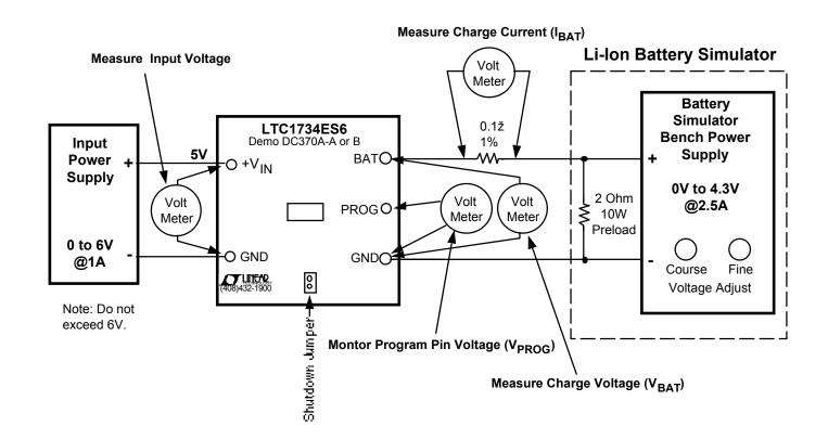
Continue slowly increasing the battery simulator power supply until the charge current drops to approximately 70mA (7mV on the charge current DVM), then read the charger output voltage on the DVM. This reading is the charger float voltage which will be either 4.1V or  $4.2V \pm 40mV$  depending on which version of the demoboard is being evaluated. The program pin voltage will indicate approximately 150mV, indicating 10% of the full programmed current.
