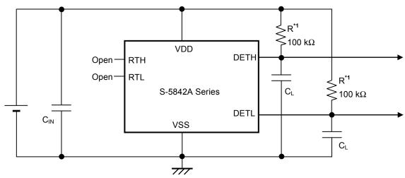
\*1. Resistor (R) is unnecessary for CMOS output product.
