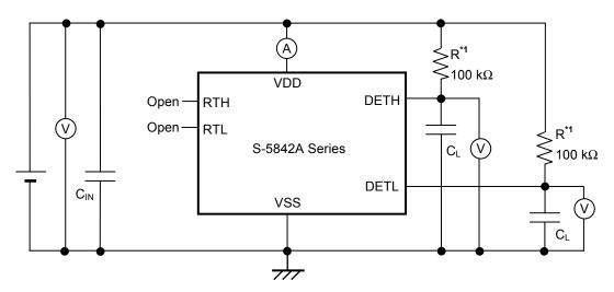
\*1. Resistor (R) is unnecessary for the CMOS output product.
