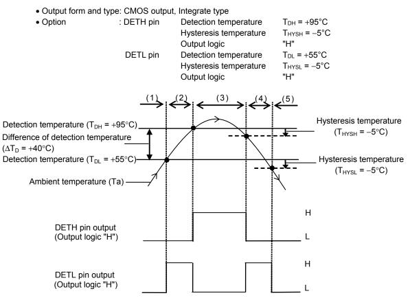
Figure 12 Timing Chart for CMOS Output and Integrate Type
