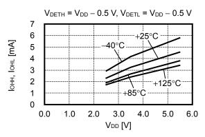
3. Output current "L" of DETH / DETL pin vs. Power supply voltage characteristics
