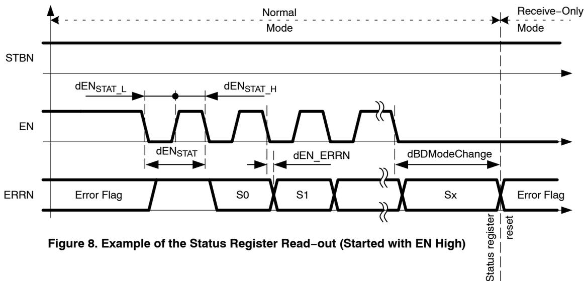
**Figure 8. Example of the Status Register Read-out (Started with EN High)**
