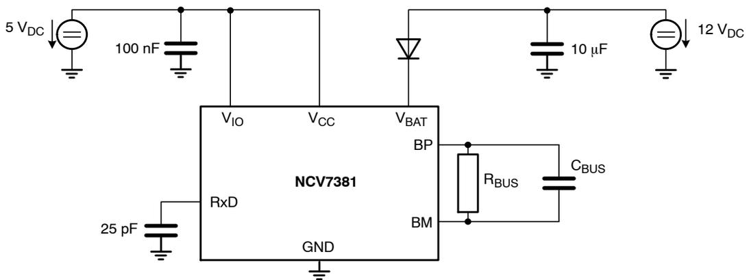
**Figure 17. Test Setup for Dynamic Characteristics**
