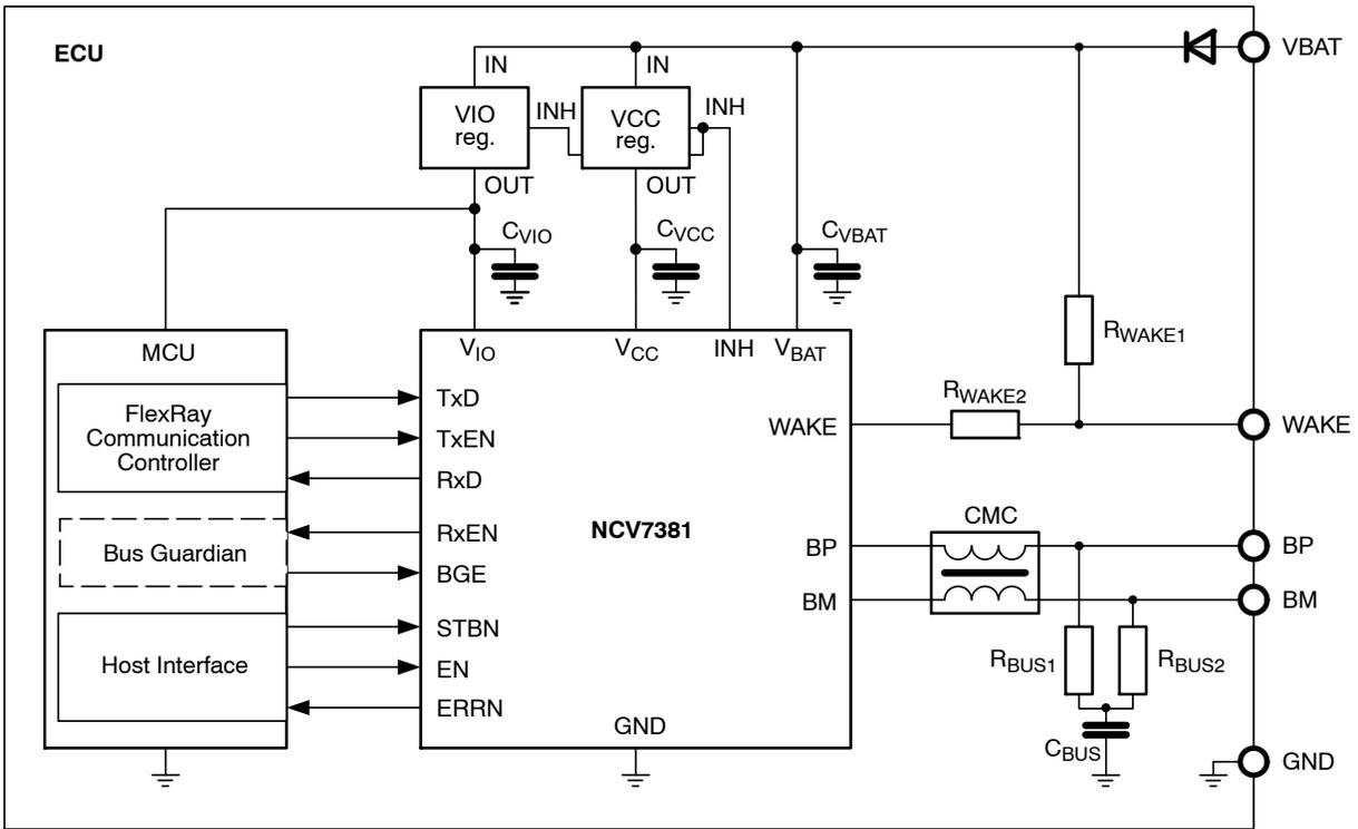
Figure 2. Application Diagram
