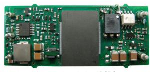
The IBC04-36S12 is the latest wide-range input isolated DCDC converter specifically designed to supply non-isolated converter architectures. It operates from an ultra-wide input range of 18 Vdc to 60 Vdc and provides a regulated output voltage of 12 V. The output is rated to a power level up to 50 W.
