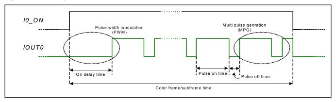
Figure 3-1. Example of PWM and MPG Timers
