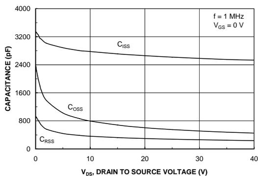
Figure 8. Capacitance Characteristics.
