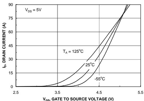
Figure 5. Transfer Characteristics.
