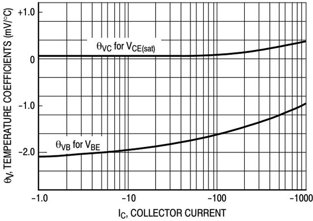
Figure 7. Temperature Coefficients
