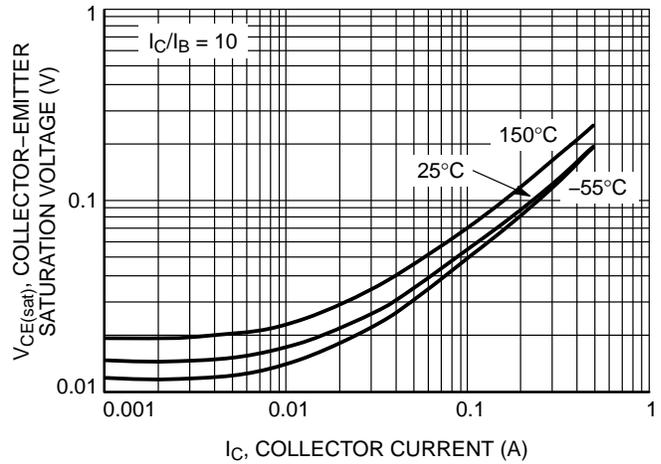
**Figure 10. Collector Emitter Saturation Voltage vs. Collector Current**
