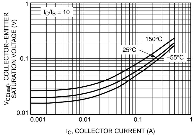
**Figure 2. Collector Emitter Saturation Voltage vs. Collector Current**
