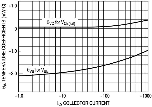
Figure 15. Temperature Coefficients
