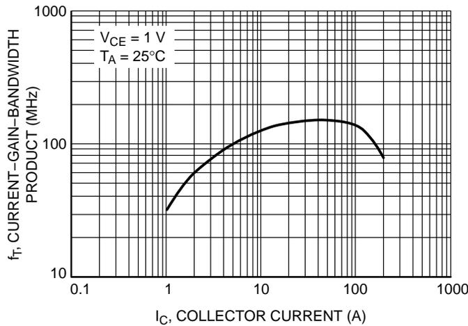
**Figure 5. Current Gain Bandwidth Product vs. Collector Current**
