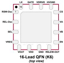
Center heat slug is at ground potential. Pads are at the bottom of the package.
