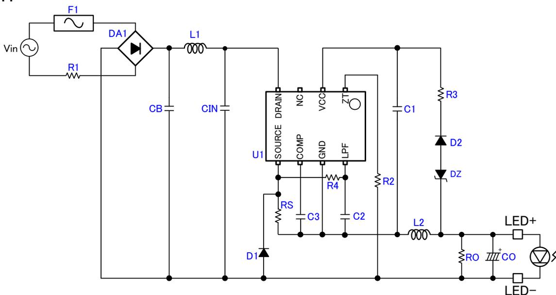
Figure 1. Application Circuit
