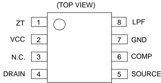
Figure 2. Pin Configuration
