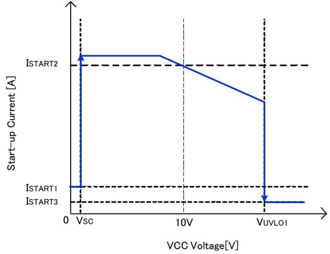
Figure 6. Start-up Current – VCC Voltage Curve
