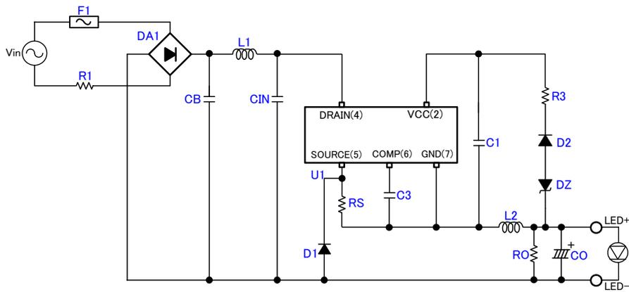
Figure 7. DC/DC Schematic
