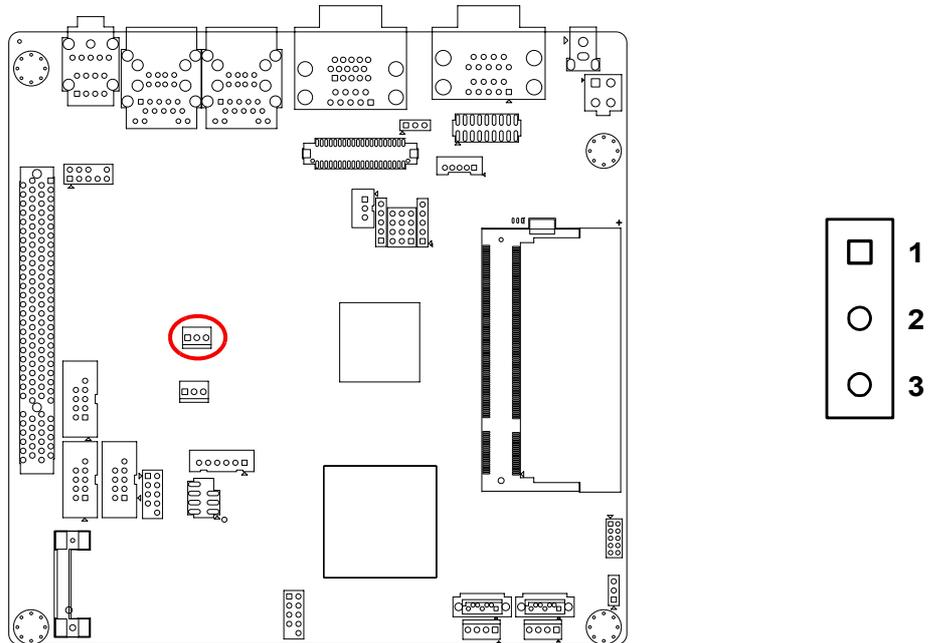
If a fan is used, this connector supports cooling fans of 500 mA (6 W) or less.
