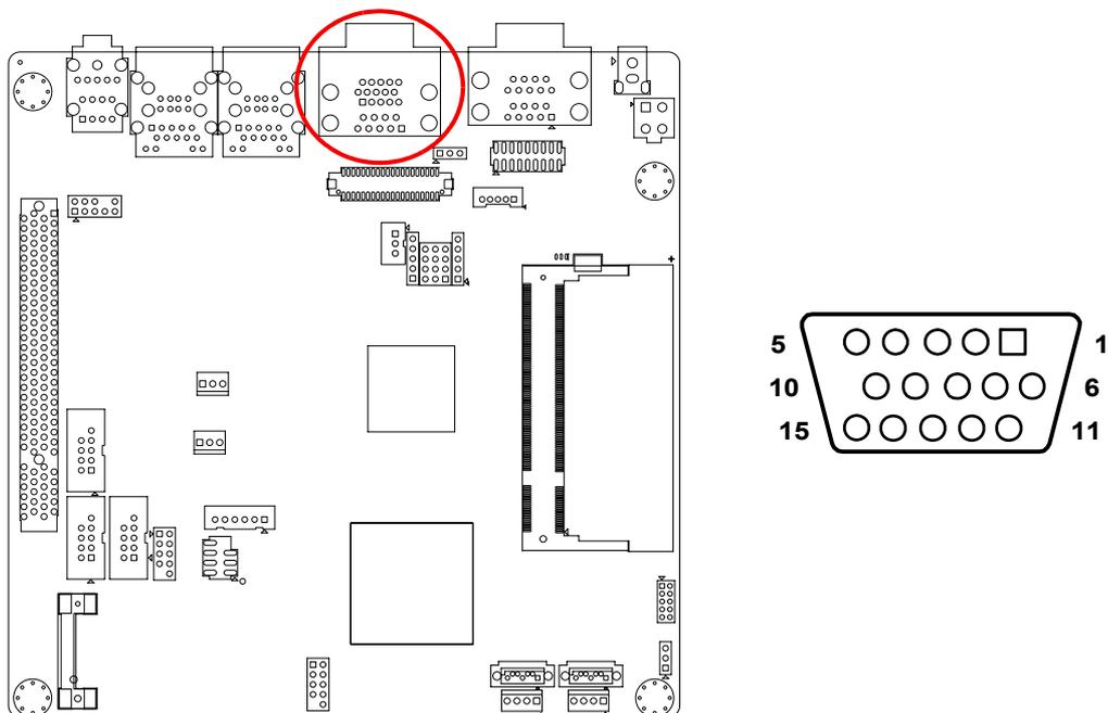
The AIMB-212 includes a VGA interface that can drive conventional CRT displays. VGA1 is a standard 15-pin D-SUB connector commonly used for VGA. Pin assignments for CRT connector VGA1 are detailed in Appendix B.
