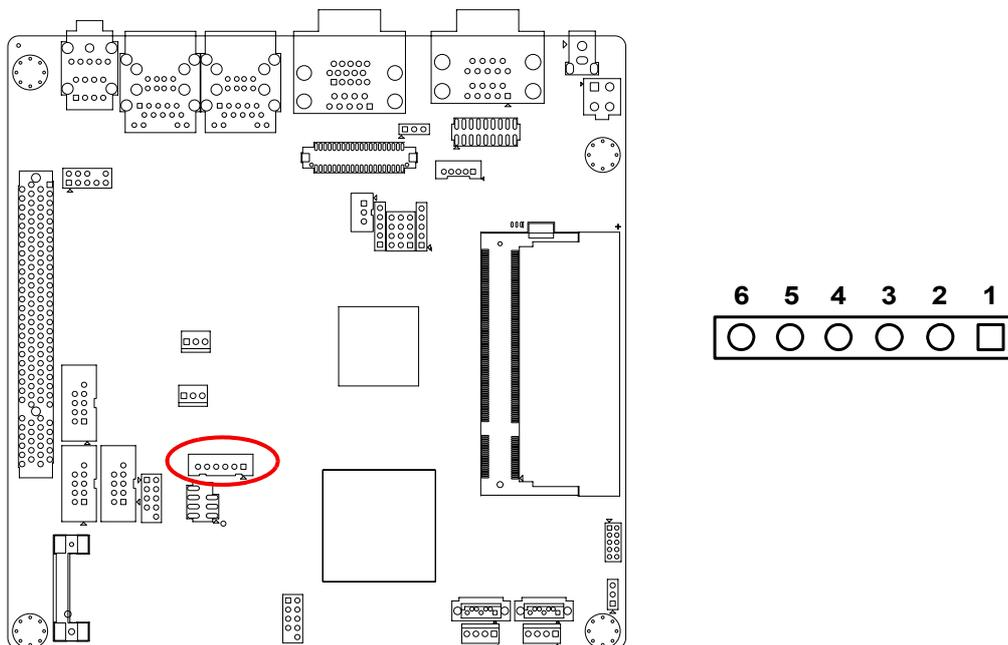
On board 6-pin wafer box connector, supports one standard PS/2 keyboard, one standard PS/2 mouse.
