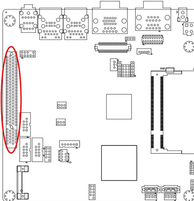
The AIMB-212 provides 1 x PCI slot.
