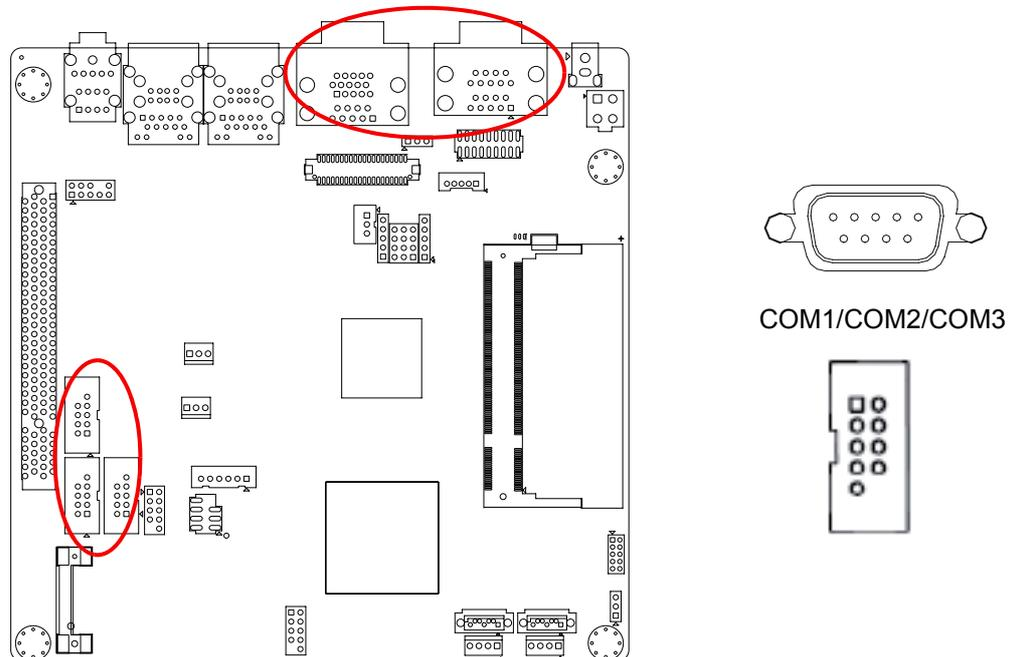
AIMB-212 supports six serial ports. 1 of RS-232/422/485 - COM1, COM2, COM3, COM4, COM5 and COM6. The user can use JSETCOM2 to select among RS 232/422/485 modes for COM2. These ports can connect to serial devices, such as a mouse or a printer, or to a communications network.
