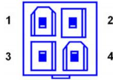
**Table B.20: ATX 12 V connector (ATX12V\_1)**
