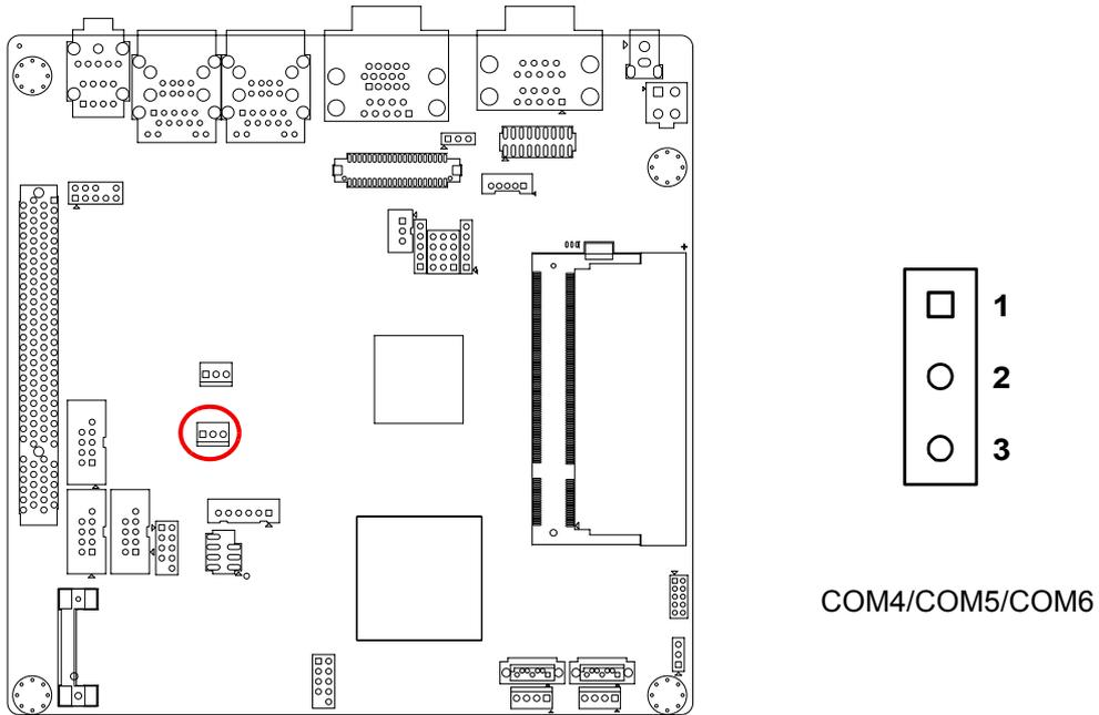
If a fan is used, this connector supports cooling fans of 500 mA (6 W) or less.
