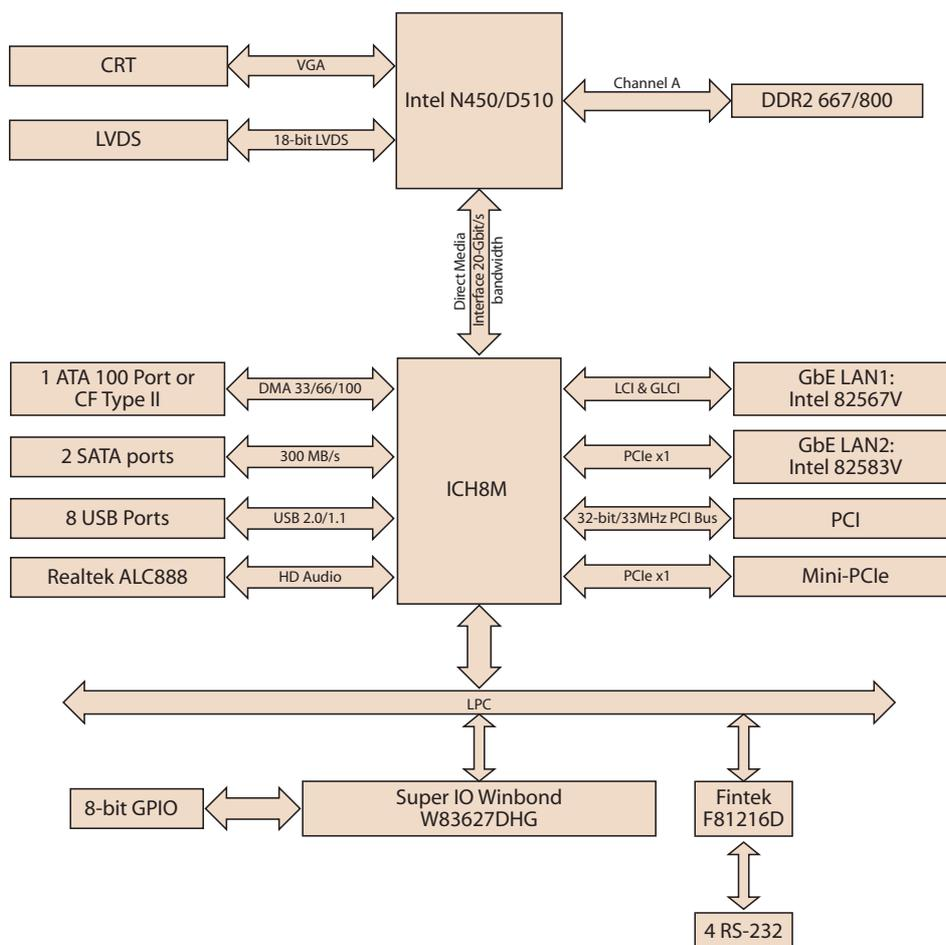
**Figure 1.3 AIMB-212 Board Diagram**
