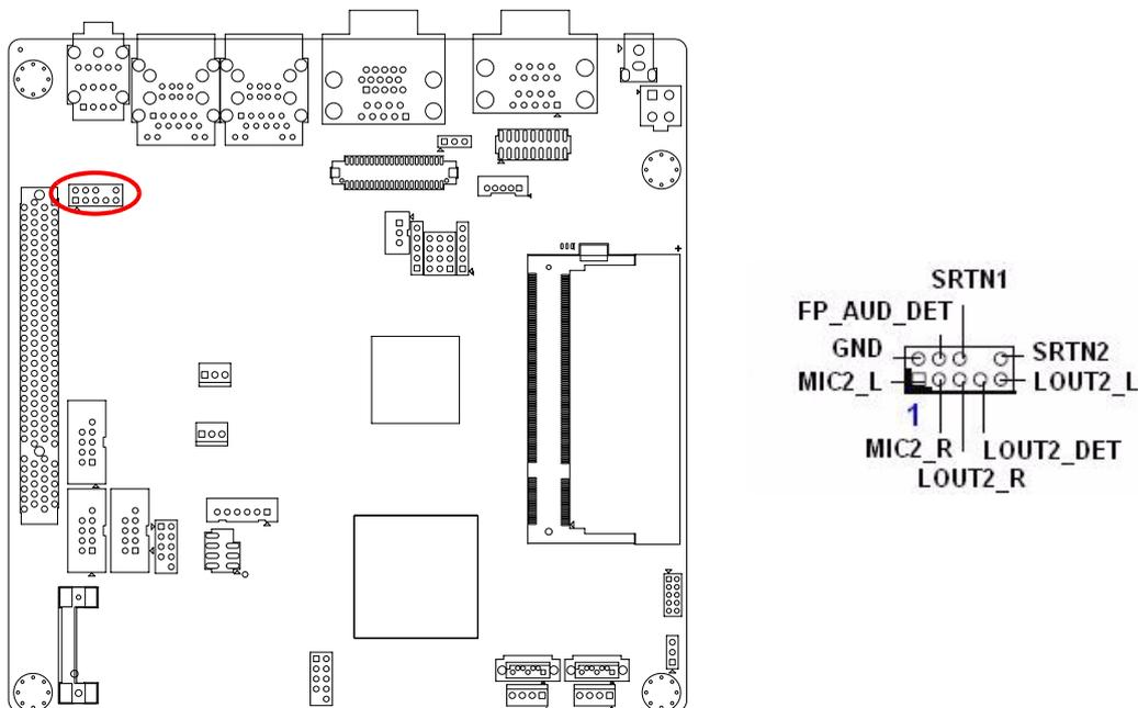
**Note!** *For motherboards with the optional HD Audio feature, we recommend that you connect a high-definition front panel audio module to this connector to take advantage of the motherboard's high definition audio capability.*
