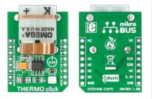
THERMO Click<sup>™</sup> is an accessory board in **mikroBUS**<sup>™</sup> form factor. It's a compact solution for adding thermocouple to your device. It features **MAX31855K** thermocouple-to-digital converter as well as **PCC-SMP** connector for K-type thermocouple probes. THERMO Click<sup>™</sup> communicates with the target board via SPI interface (Read-only). The board is designed to use 3.3V power supply only. It has a LED diode (GREEN) that indicates the presence of power supply.
