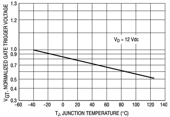
Figure 4. Typical Gate Trigger Voltage versus Temperature
