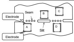
\*1 A > D is valid when stress is added vertically to the perforation as with Hand Separation. If a Cutting Disc is used, stress will be diagonal to the PCB, therefore A > D is invalid.
