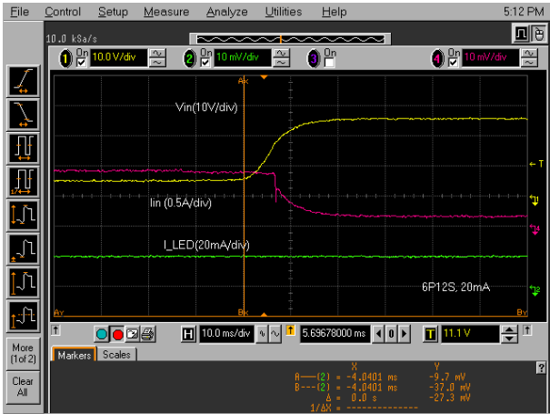
FIGURE 14. LINE REGULATION WITH V_{IN} CHANGE FROM 6V TO 26V, V_{IN} = 12V , 4P12S AT 20mA/CHANNEL
