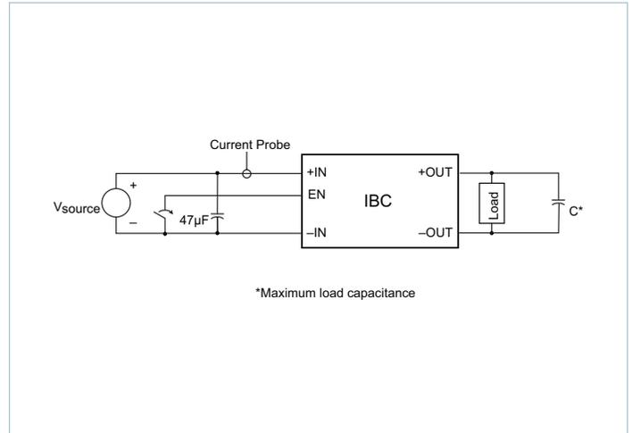
Figure 22 — Test circuit; inrush current overshoot
