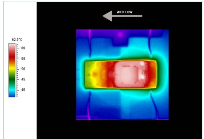
**Figure 28** — Thermal plot, 400LFM, 25°C, 48V<sub>IN</sub>, 300W output power
