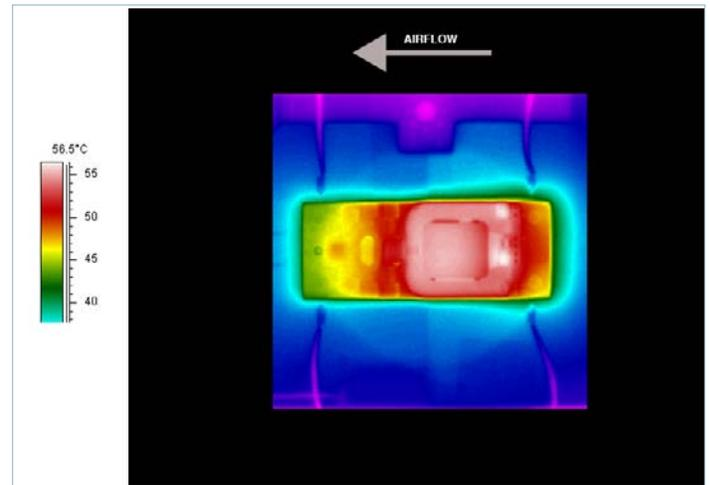
**Figure 30** — Thermal plot, 600LFM, 25°C, 48V<sub>IN</sub>, 300W output power
