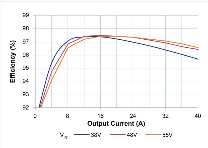
Figure 3 — Efficiency vs. output current, 70°C ambient
