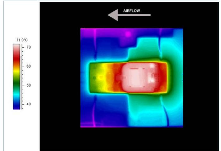
**Figure 26** — Thermal plot, 200LFM, 25°C, 48V<sub>IN</sub>, 300W output power
