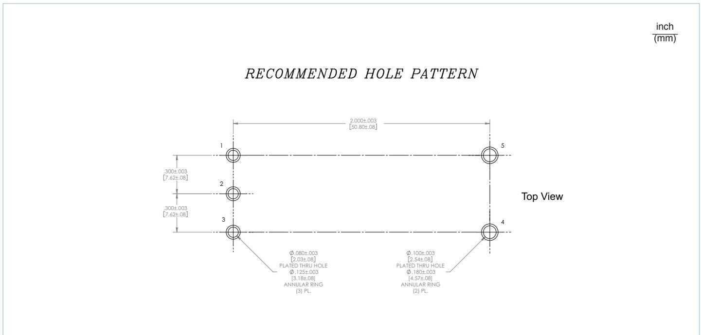
Figure 33 — IBC PCB recommended hole pattern
