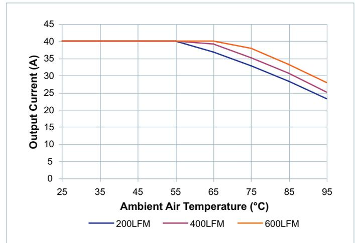
**Figure 20** — Output current derating vs. ambient air temperature at  $V_{IN}$  nominal. Longitudinal airflow. Board and junction temperatures within IPC-9592 derating guidelines
