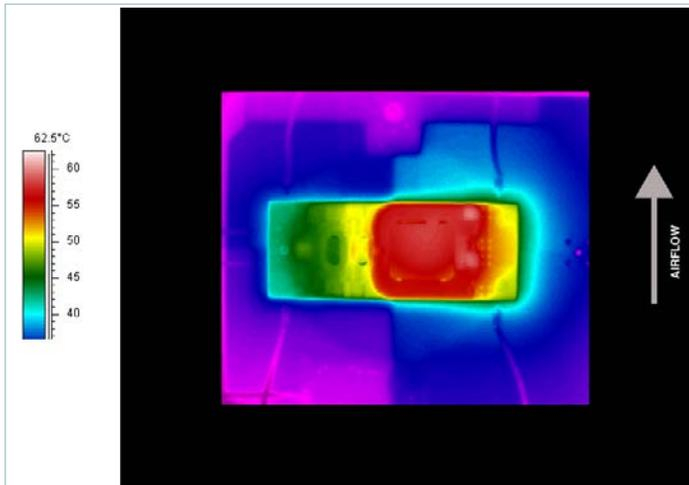
**Figure 27** — Thermal plot, 400LFM, 25°C, 48V<sub>IN</sub>, 300W output power
