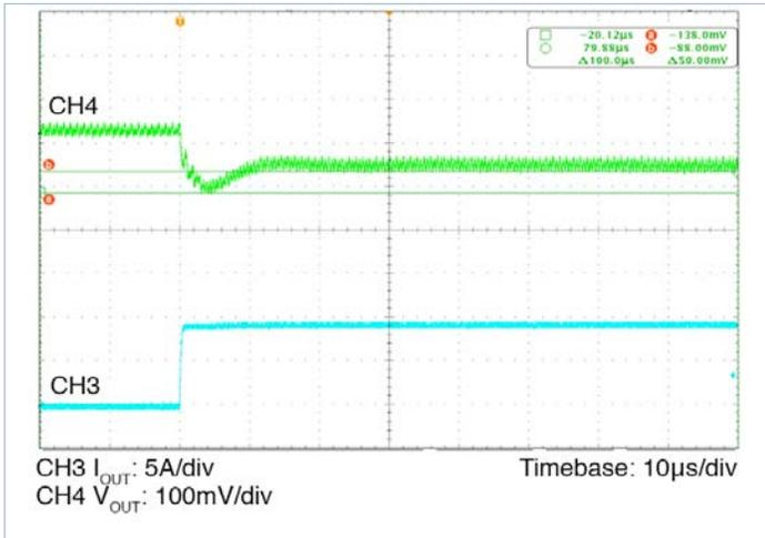
Figure 11 — Load transient response; nominal line Load step 75–100%
