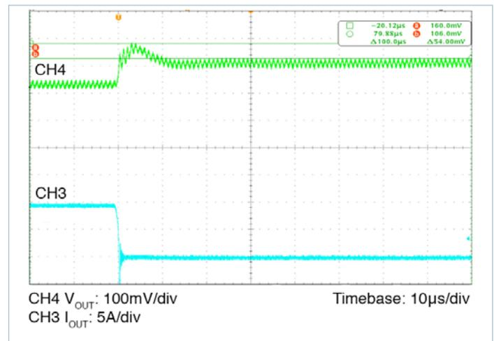
Figure 14 — Load transient response; nominal line Load step 25–0%
