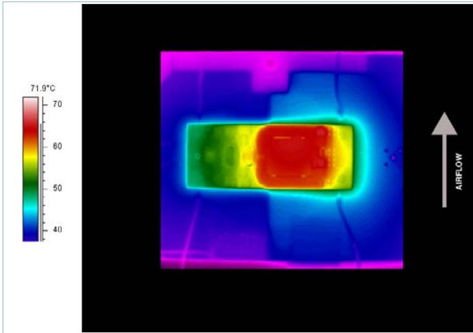
**Figure 25** — Thermal plot, 200LFM, 25°C, 48V<sub>IN</sub>, 300W output power
