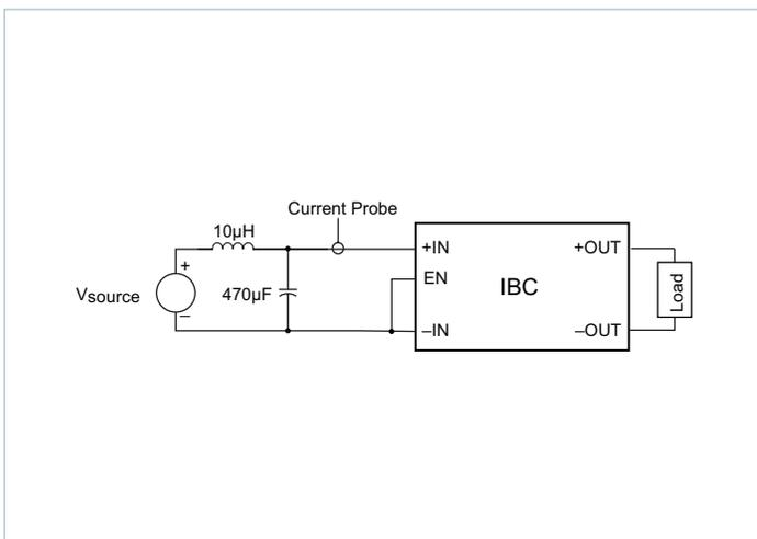
Figure 23 — Test circuit; input reflected ripple current
