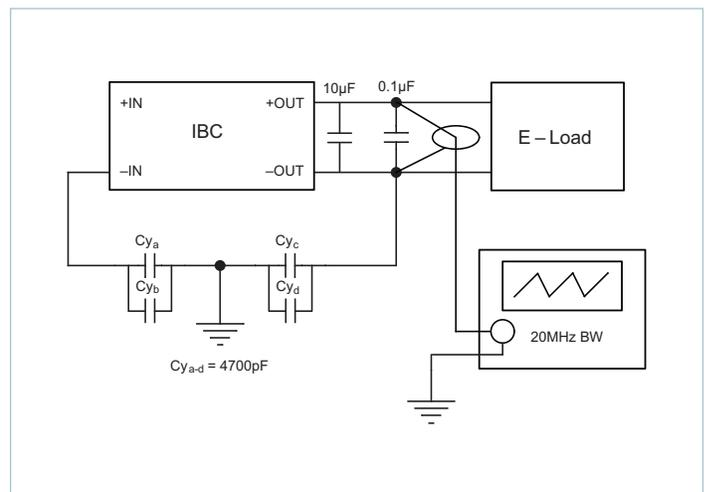
Figure 24 — Test circuit; output voltage ripple
