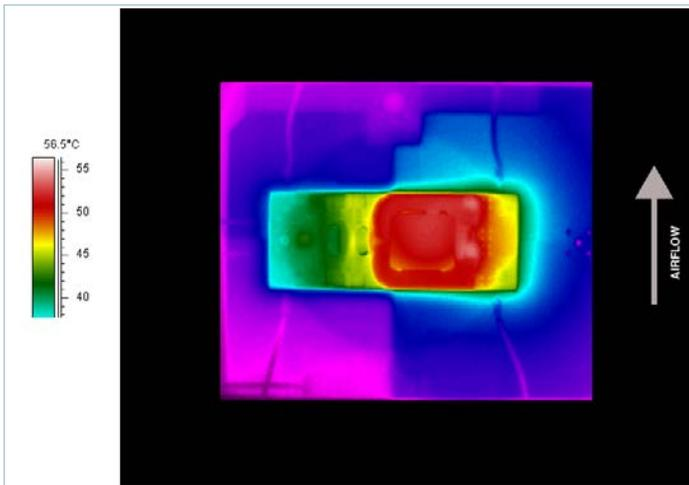
**Figure 29** — Thermal plot, 600LFM, 25°C, 48V<sub>IN</sub>, 300W output power
