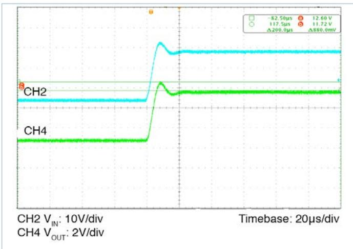
Figure 15 — Input transient response; V<sub>IN</sub> step low line to high line at full load
