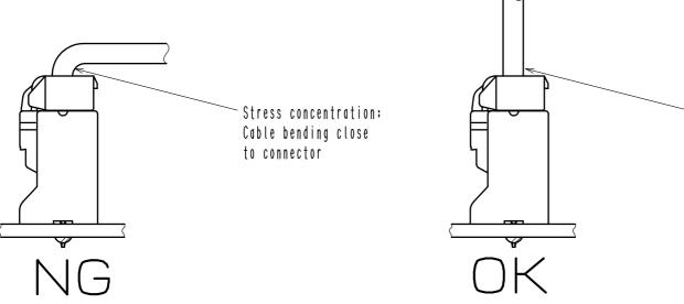
2) When applying load to connector end, please use the retainer for reducing the stress affection on the connector. Retainer shall be installed after inserted crimping contact completely. It might be impossible to insert it when terminal installation is incompleted.
