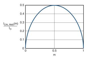
Figure 3. I<sub>CIN</sub> vs. Voltage Conversion Ratio
