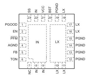
23-Pin 4mm x 4mm QFN (Top View)
