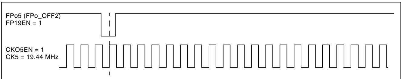
Figure 12 - Output Timing for CKo5 and FPo5 (FPo\_OFF2)
