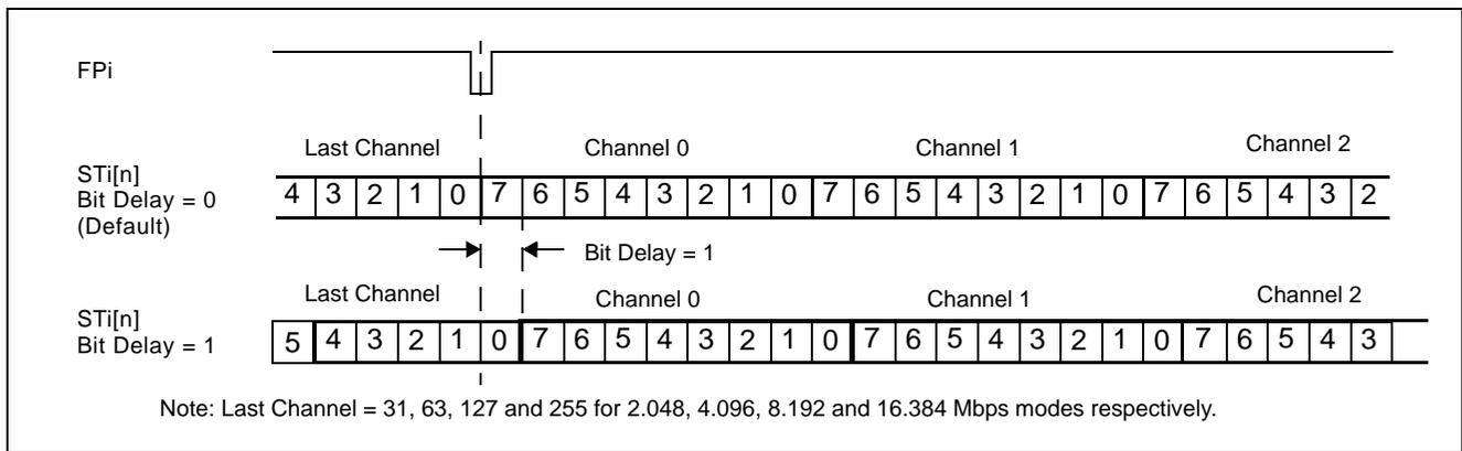
Figure 13 - Input Bit Delay Timing Diagram (ST-BUS)
