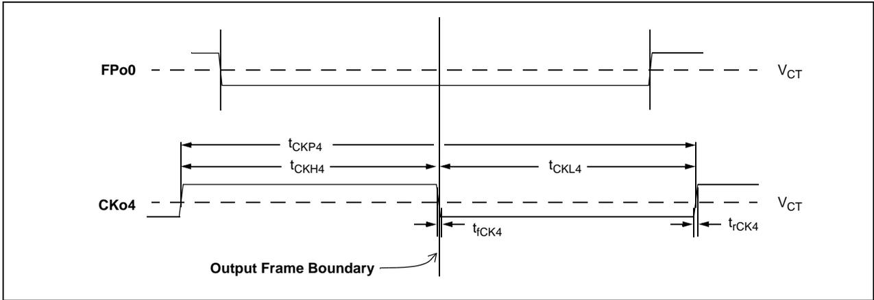
Figure 46 - FPo4 and CKo4 Timing Diagram (1.544/2.048 MHz)
