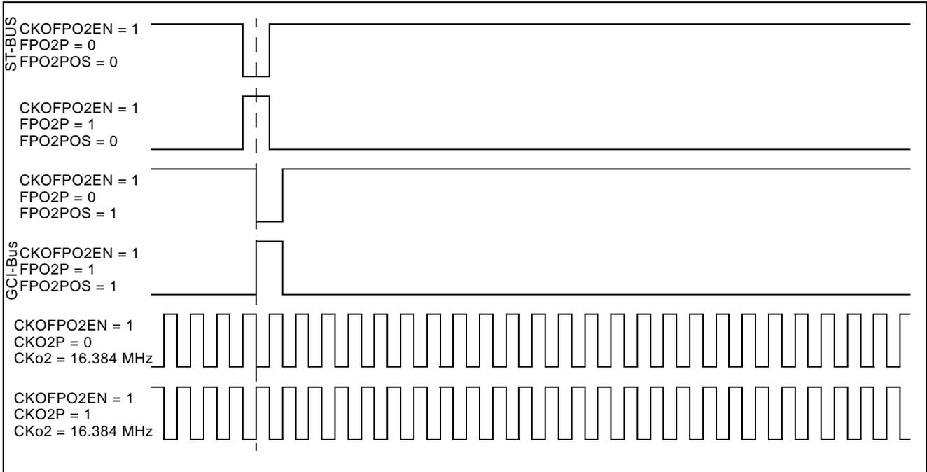
Figure 9 - Output Timing for CKo2 and FPo2
