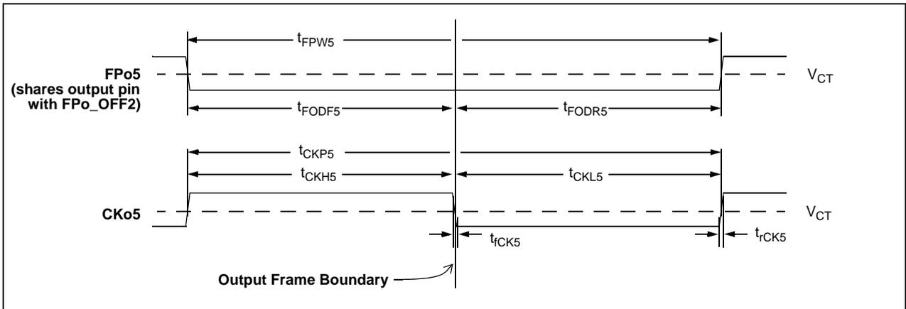
Figure 47 - CKo5 Timing Diagram (19.44 MHz)
