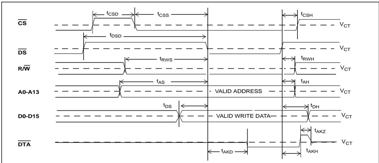
**Figure 27 - Motorola Non-Multiplexed Bus Timing - Write Access**
