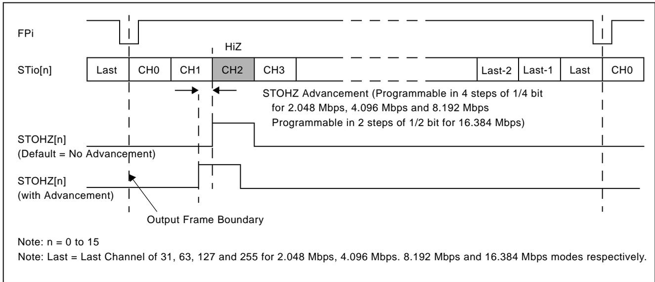
Figure 18 - Channel Switching External High Impedance Control Timing
