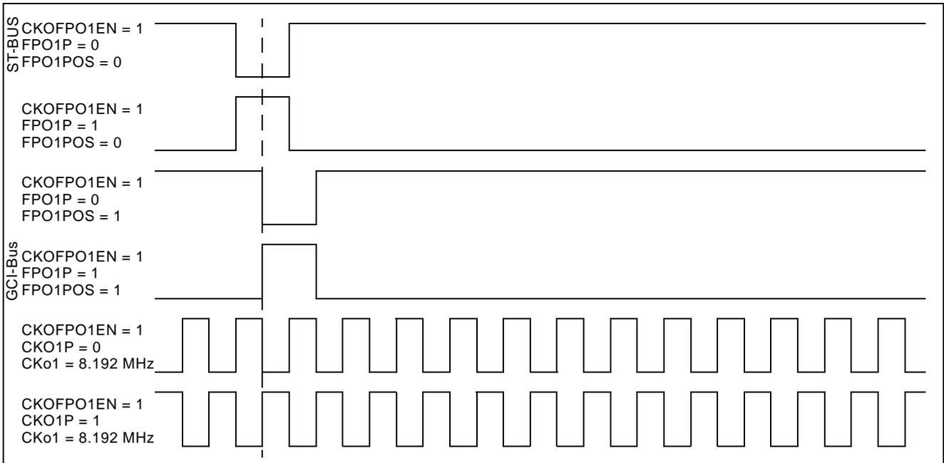
Figure 8 - Output Timing for CKo1 and FPo1
