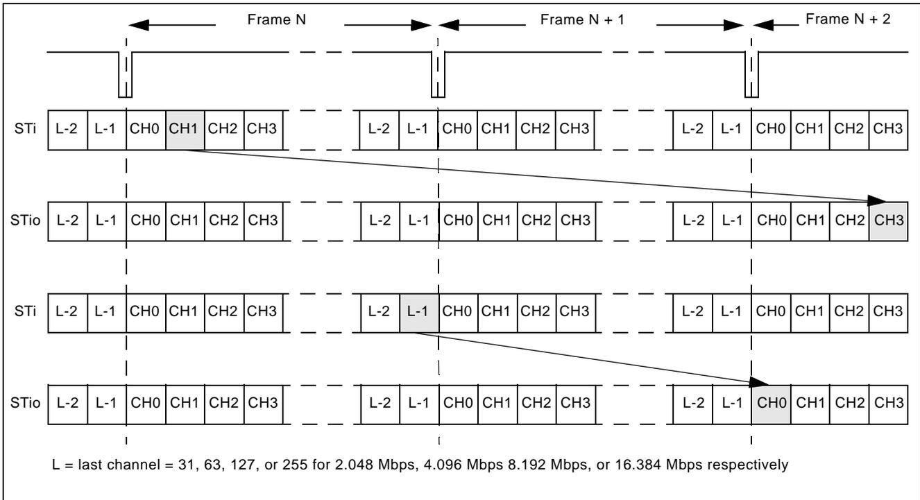
Figure 20 - Data Throughput Delay for Constant Delay
