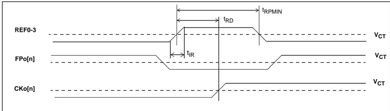
**Figure 48 - REF0 - 3 Reference Input/Output Timing**
