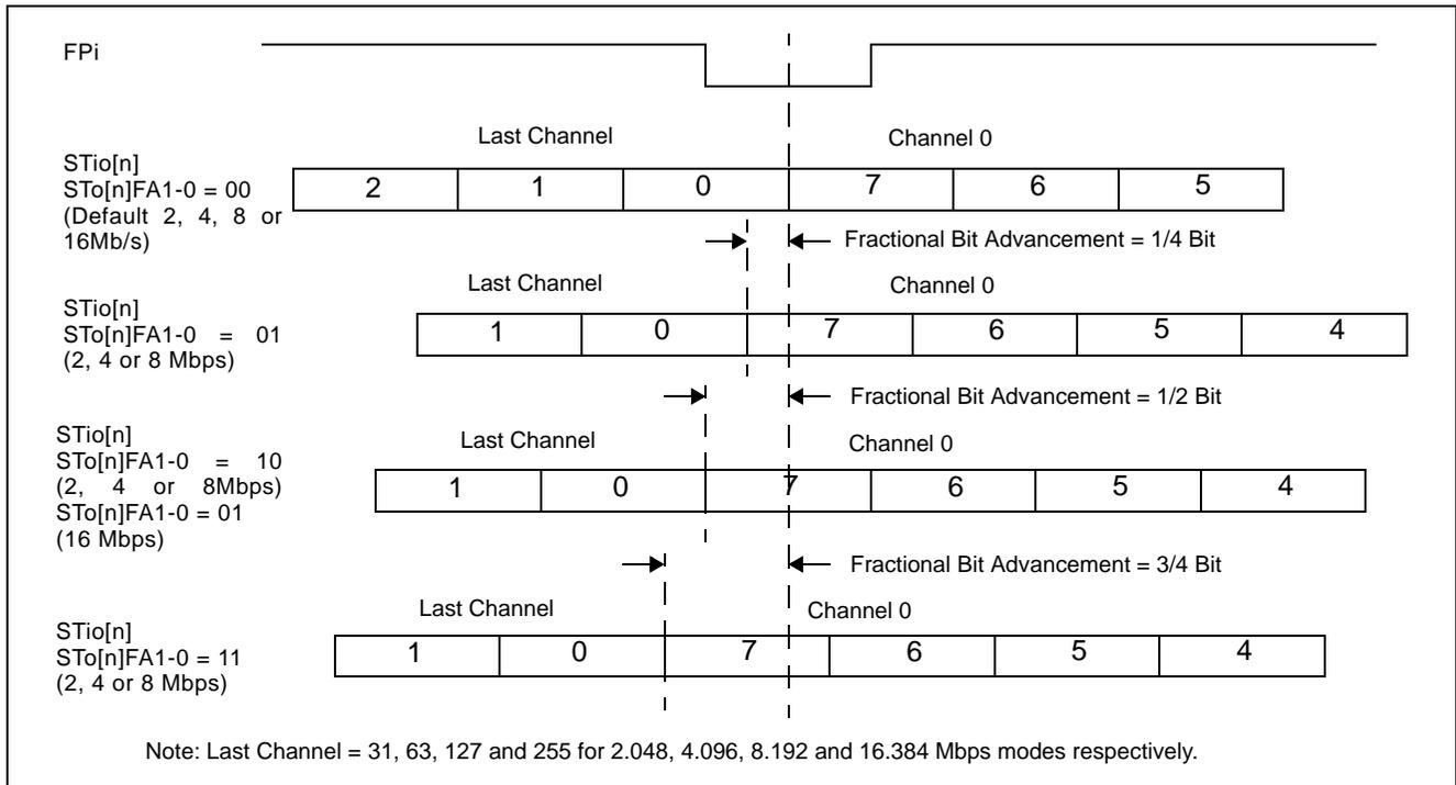
Figure 17 - Output Fractional Bit Advancement Timing Diagram (ST-BUS)
