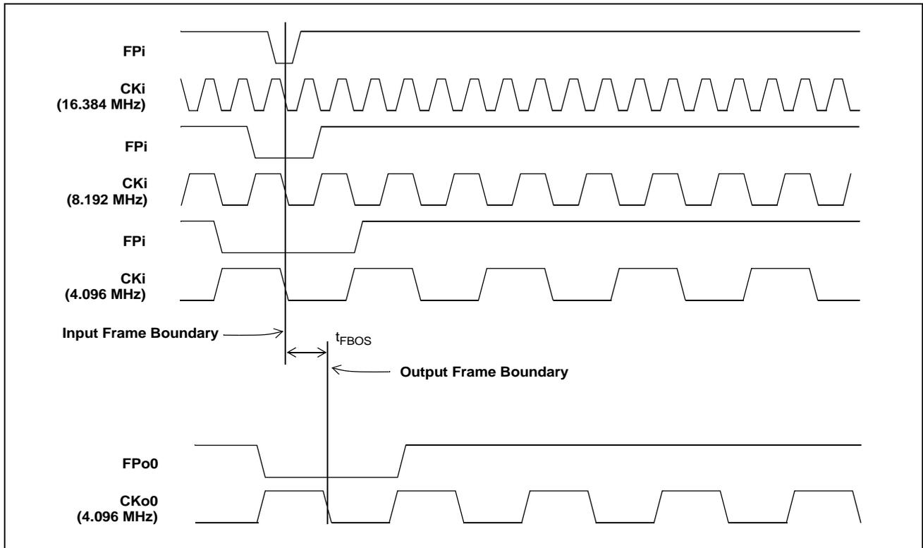
**Figure 41 - Input and Output Frame Boundary Offset**
