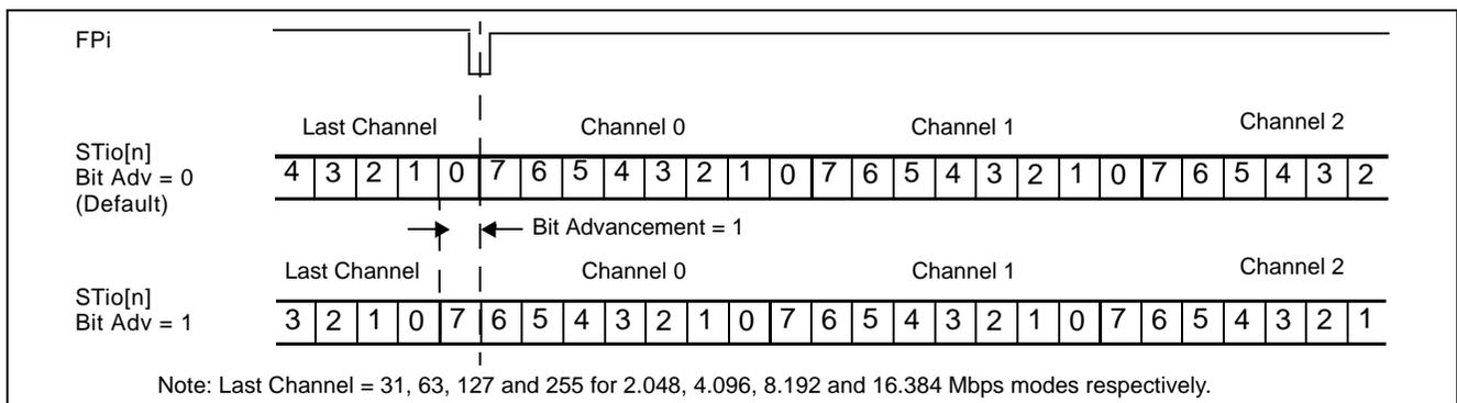
Figure 16 - Output Bit Advancement Timing Diagram (ST-BUS)
