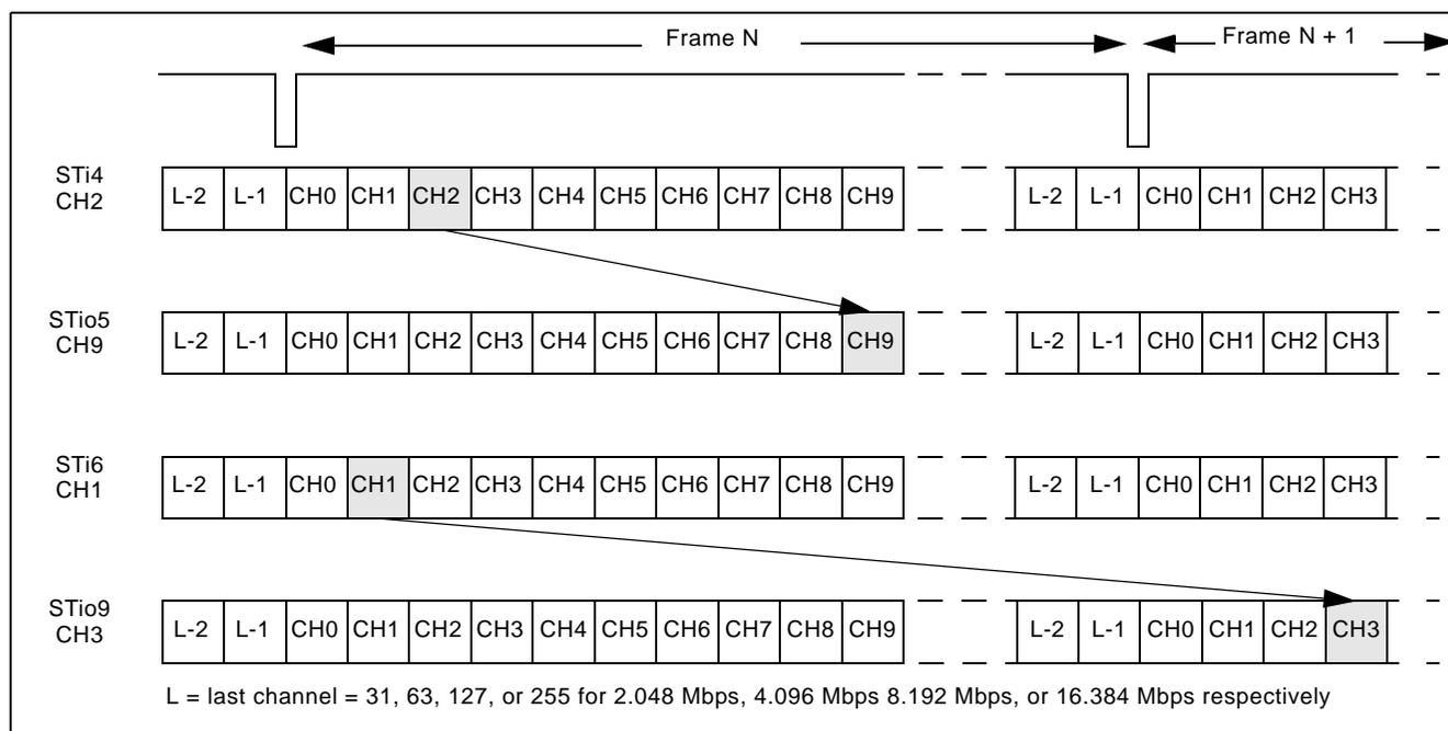
**Figure 19 - Data Throughput Delay for Variable Delay**
