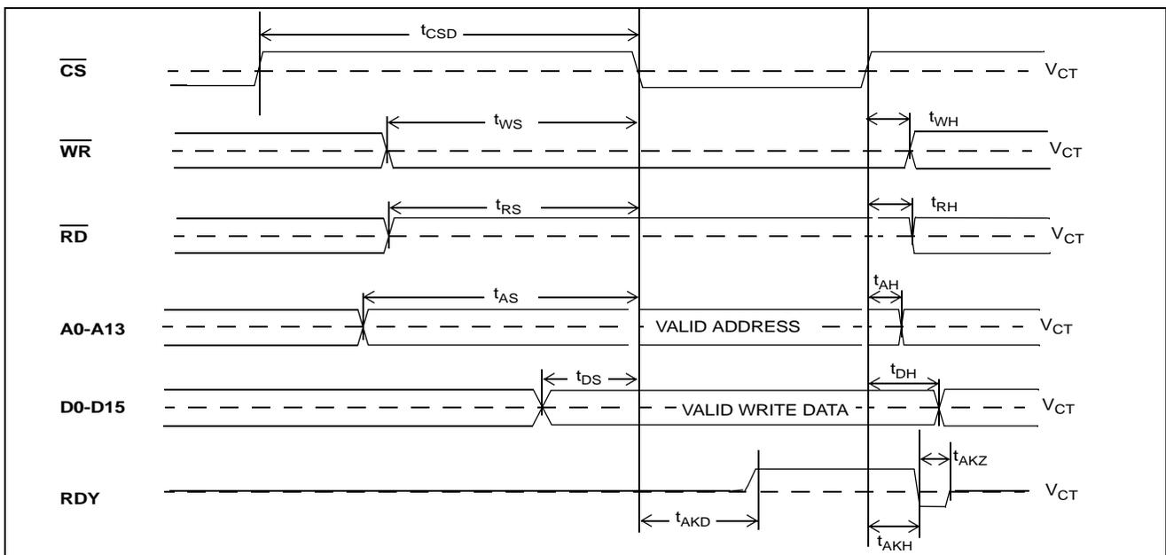
**Figure 29 - Intel Non-Multiplexed Bus Timing - Write Access**
