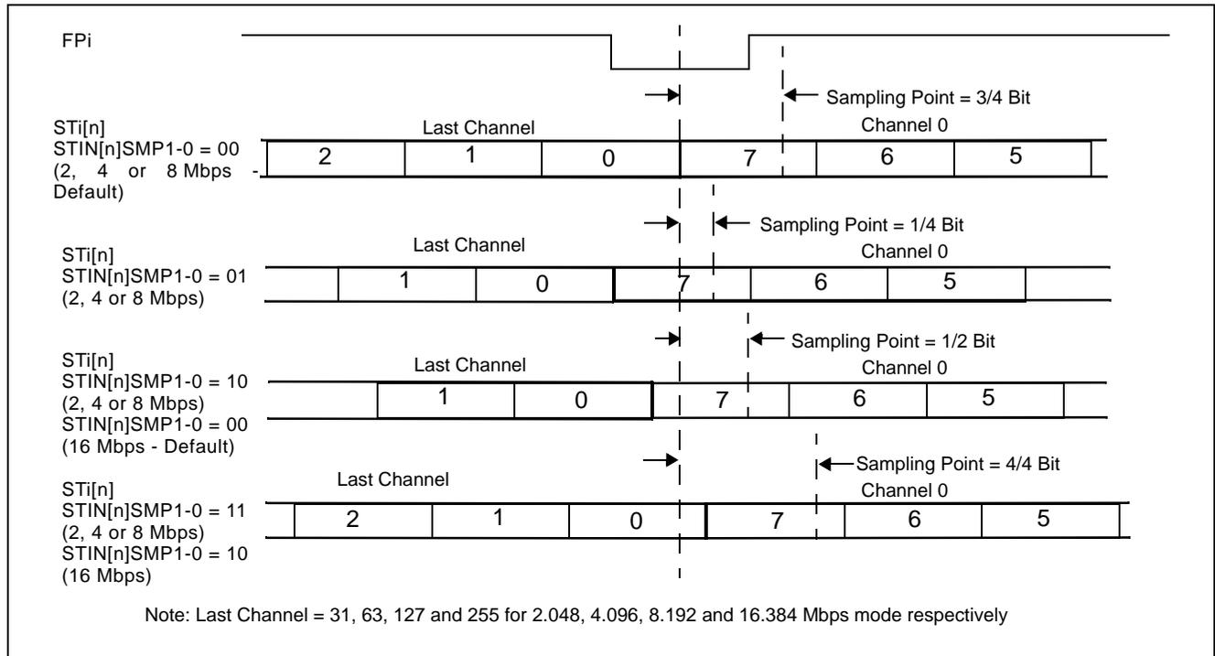
Figure 14 - Input Bit Sampling Point Programming
