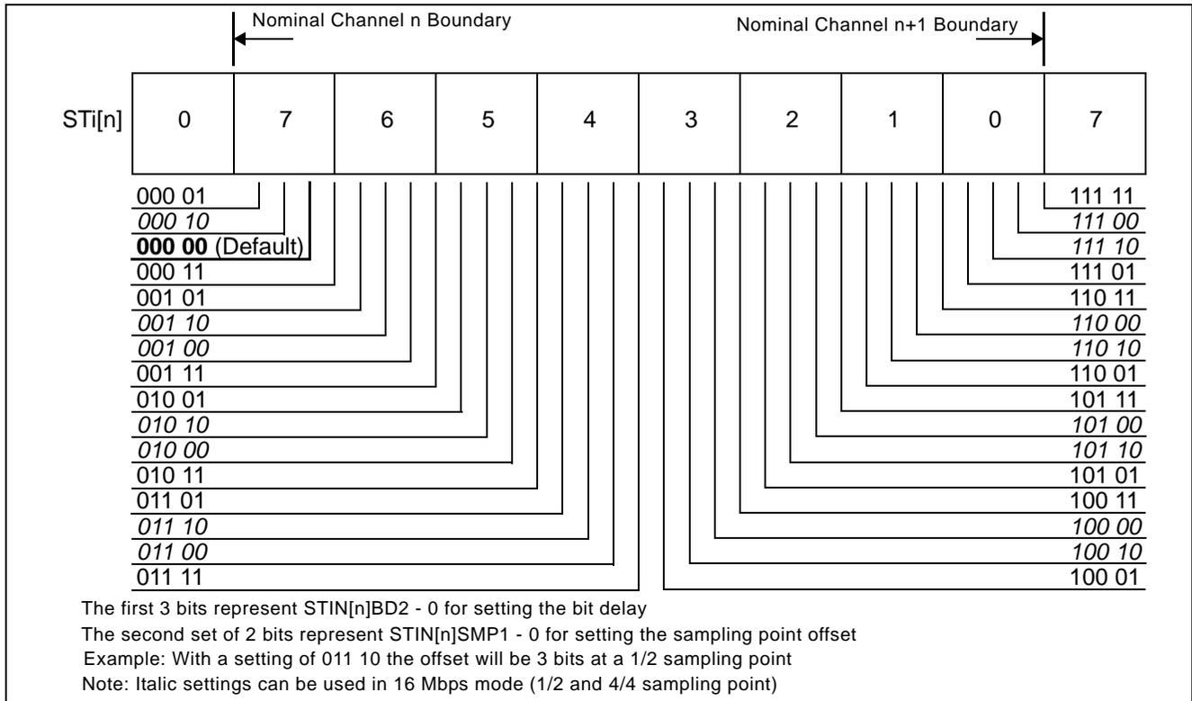
Figure 15 - Input Bit Delay and Fractional Sampling Point
