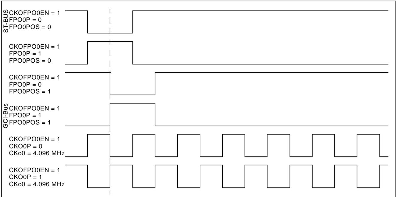
Figure 7 - Output Timing for CKo0 and FPo0
