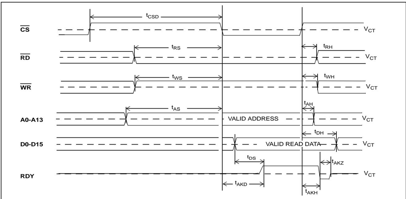
**Figure 28 - Intel Non-Multiplexed Bus Timing - Read Access**
