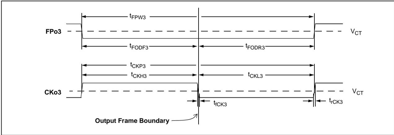
Figure 45 - FPo3 and CKo3 (32.768 MHz) Timing Diagram
