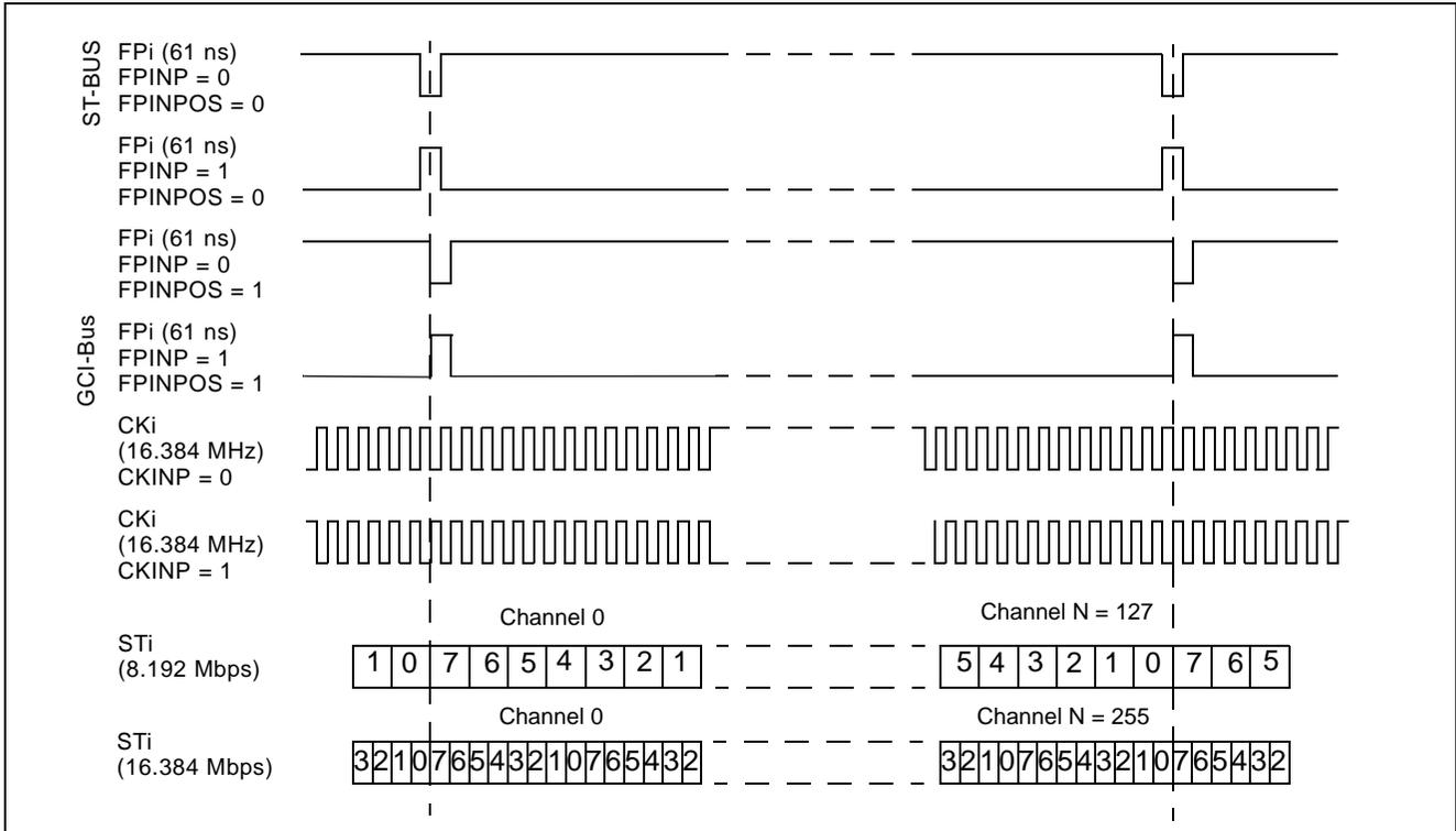
Figure 6 - Input Timing when CKIN1 - 0 = "00" in the CR
