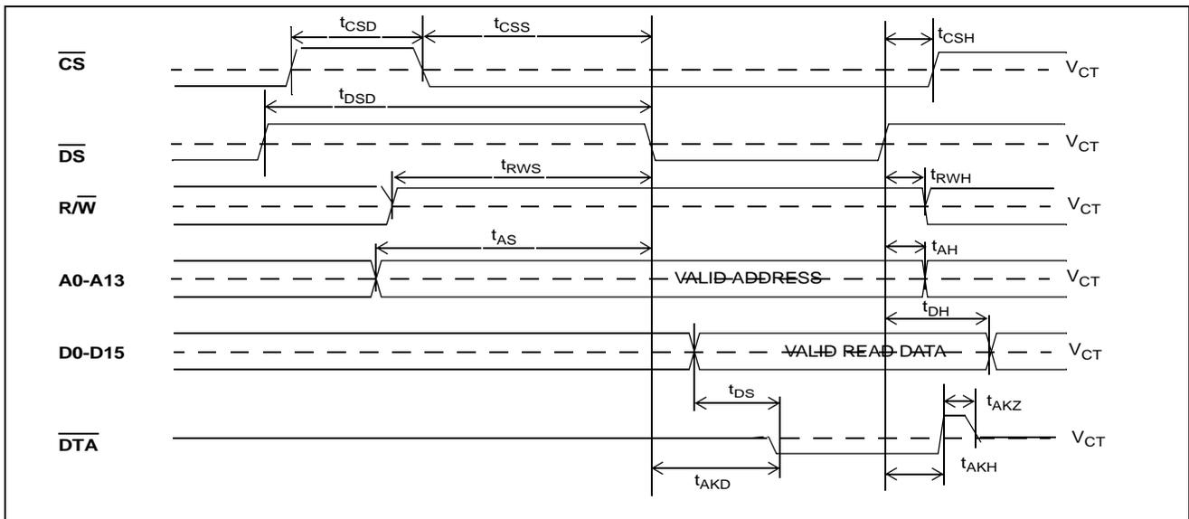
**Figure 26 - Motorola Non-Multiplexed Bus Timing - Read Access**
