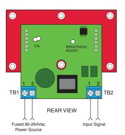
Figure 1. DMU-30DCV wiring diagram
