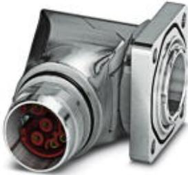
Device connector, front mounting, angled rotatable, SPEEDCON locking, M17, Number of positions: 8, Type of contact: Socket, Crimp connection, Axial O-ring, 4x Ø3.2, shielded: yes, Flange dimensions: 25.75 mm x 25.75 mm
