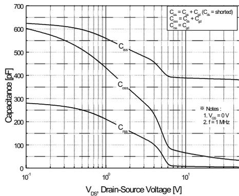
Figure 5. Capacitance Characteristics
